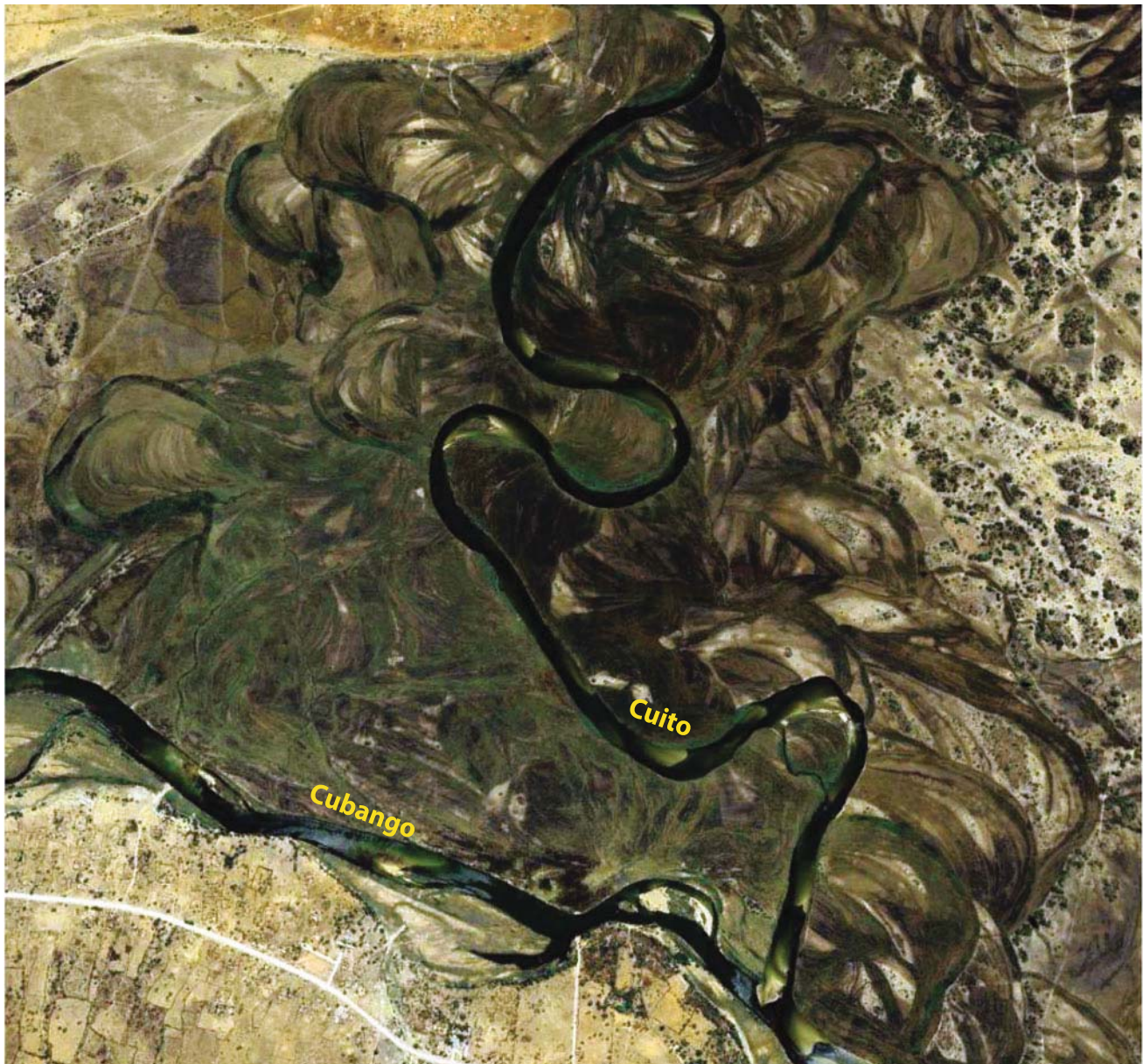
Fig. 2.14 The confluence of the Cuito and Cubango rivers on the border between Angola and Namibia. The sluggish, meandering Cuito is flanked by multiple scroll bars and oxbows, unlike the Cubango with its faster, more direct flow (image from Microsoft Bing Maps Imagery Services)
