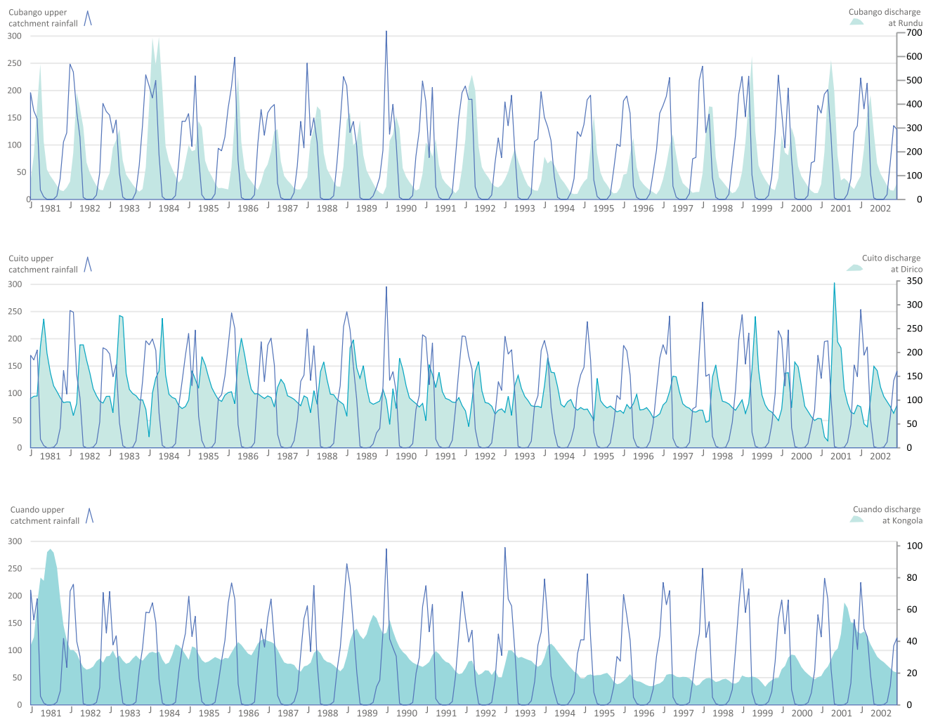
Fig. 2.23 Discharges in cubic metres per second along the Cubango (at Rundu), the Cuito (at Dirico) and Cuando (at Kongola) between 1981 and 2002, and average monthly rainfall in their upper catchments. Note the different scales of the y-axis. Each year runs from January to
