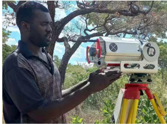
Hermane Diesse operating the terrestrial laser scanner provided by the University of Edinburgh at Kanovlei state forest.
