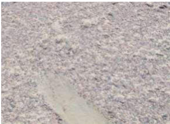
The scuff mark shows how the gravel / stones are concentrated in a thin surface layer (MC)
