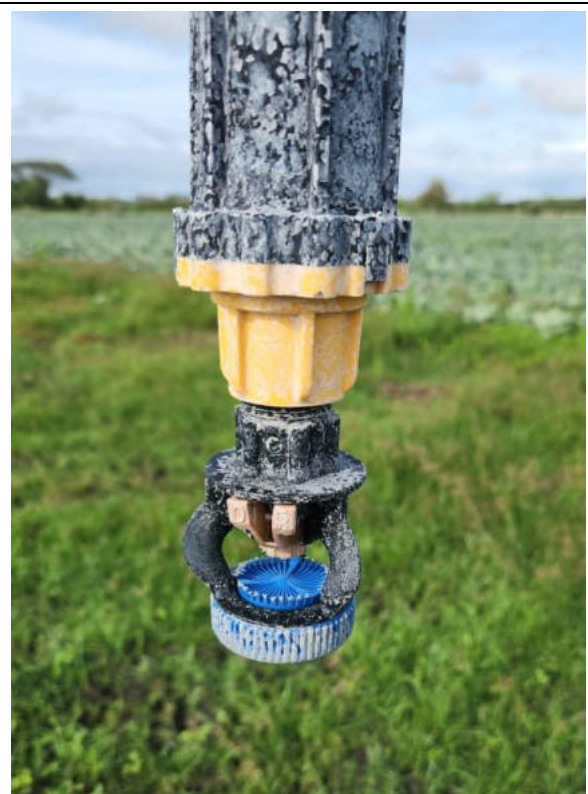
Photo 5-2 Lieper Sprinkler emitter employed by the Proponent (photo: A Blume)
