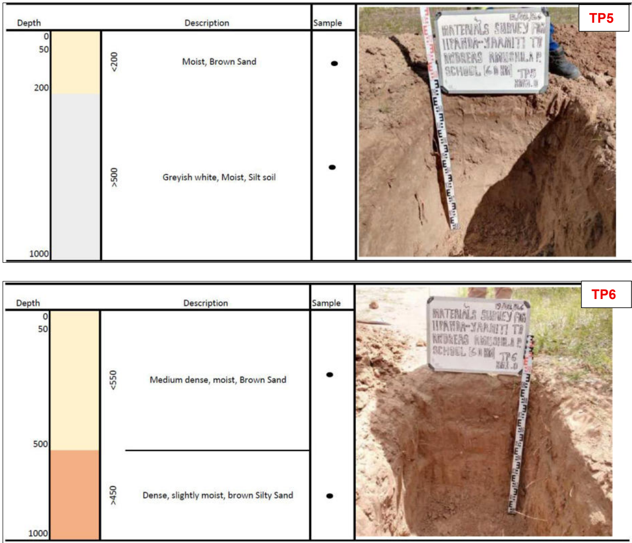
Figure 2-2: Centreline soil profiles photos of the 6 test pit sites between lipanda YaAmiti Settlement and Andreas Amushila Primary School (source: Gabriel, 2026)
