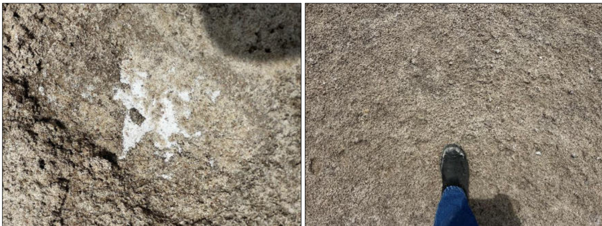
Figure 5-14: Site soils overlain by sand and gravel influenced by salt crystals
