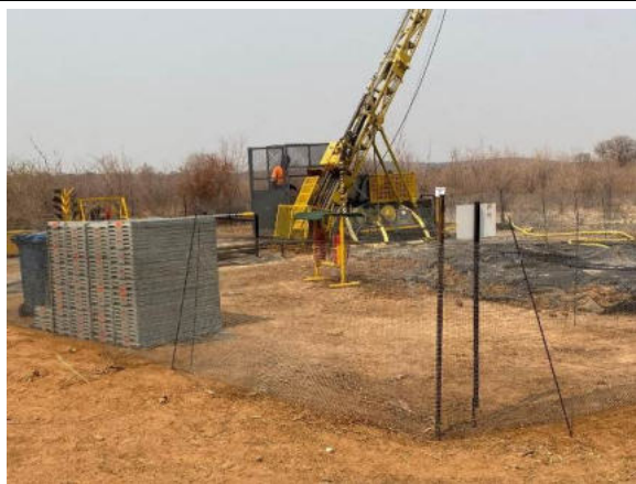
Photo 4-5 Example of core drilling operation (Votorantim site)
