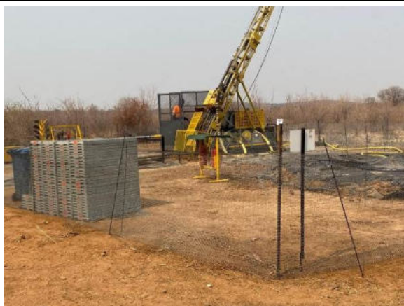
Photo 4-5 Example of core drilling operation (Votorantim site)
