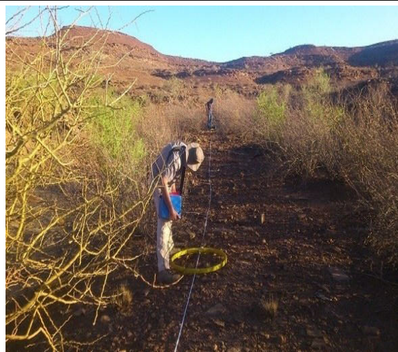
Photo 4-2 Example of a geophysical survey
