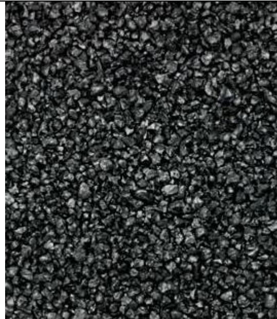
Photo 4-10 Copper slag often used for blasting
