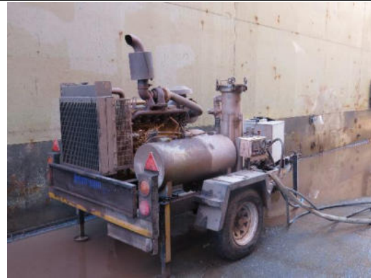
Photo 4-8 Compressor for freshwater pressurized cleaning
