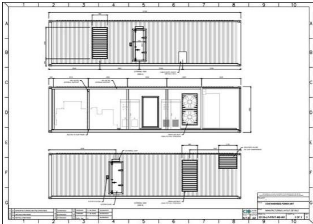
Figure 8: Genset container and layout (2)
