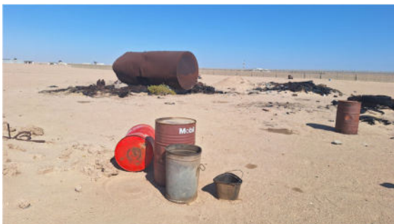
Photo 3-5 Fuel storage for training with staining
