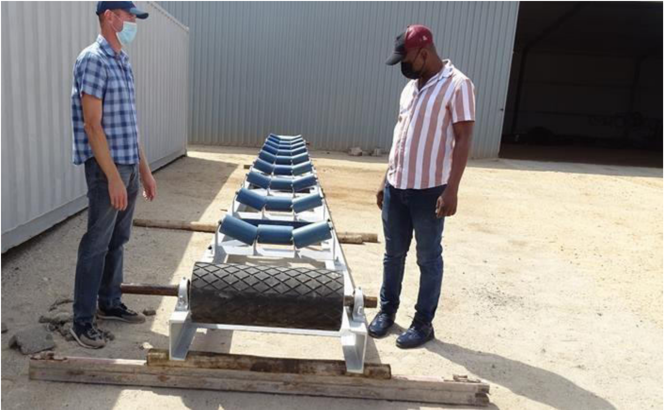
Photo 16: Under construction the conveyor to be used on the refurbished hopper feeder.
