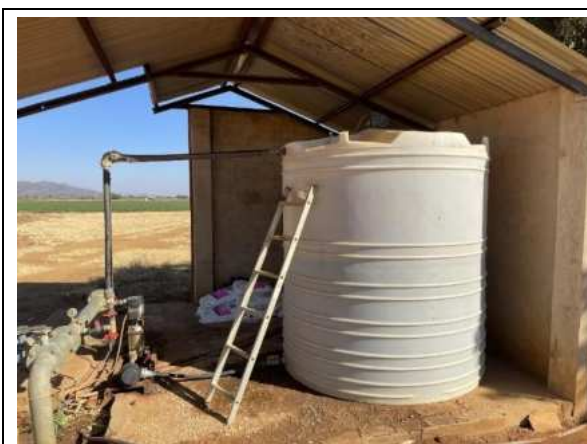
Photo 4-15 Fertiliser mixing tank
