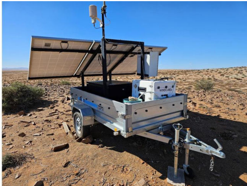
Figure 2-4: Typical LiDAR Temporary Installation (Option 2) for PML04 (source: GEO-NET, 2025)
