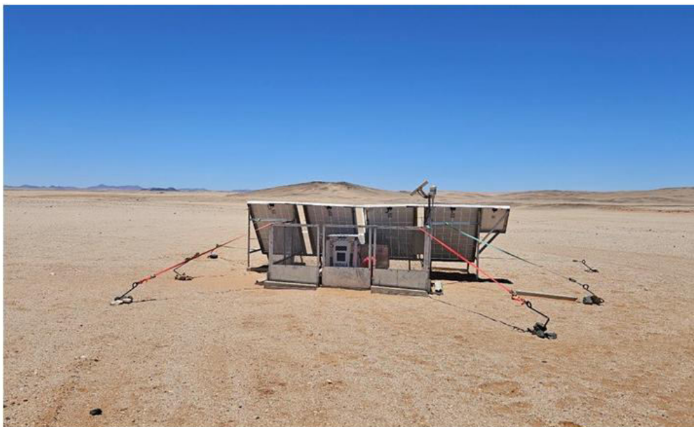
Figure 2-2: Photo of typical LiDAR Installation (Option 1) for PML04 (source: GEO-NET, 2025)
