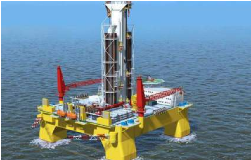
FIGURE 3-2 EXAMPLE OF SEMI-SUBMERSIBLE DRILLING UNIT
