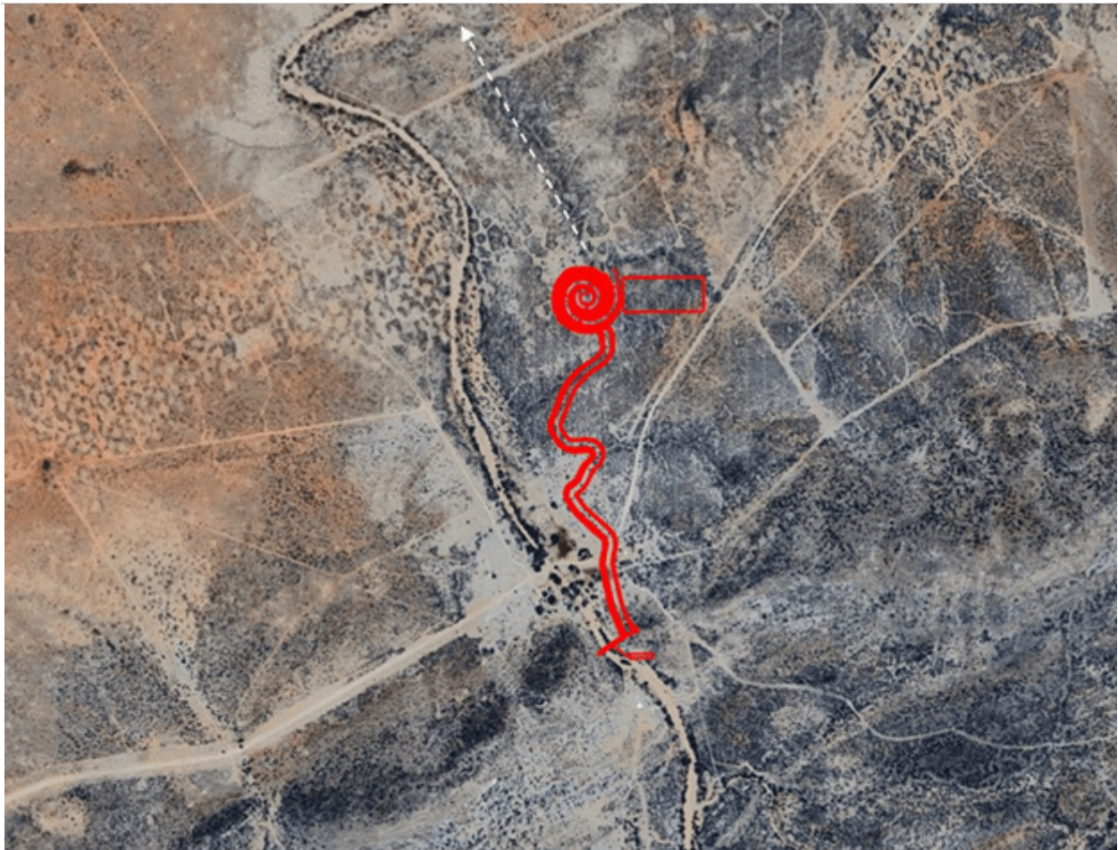
Figure 97 - Okawayo River diversion and embankment dam site. The white dashed arrow indicates the proposed direction of flow of the Okawayo River rather than damming it into the proposed holding dam (Source: (Cunningham, 2023)).
