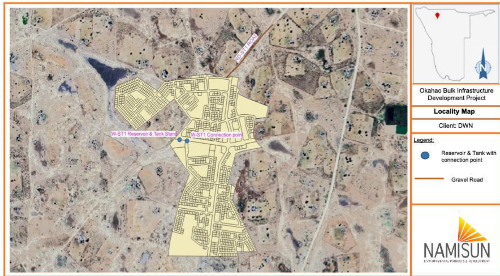
FIGURE 4: W-ST1 THE BLUE DOTS SHOW THE GROUND LEVEL RESERVOIR AND ELEVATED TANK WITH CONNECTION POINT (REF. LCE)
