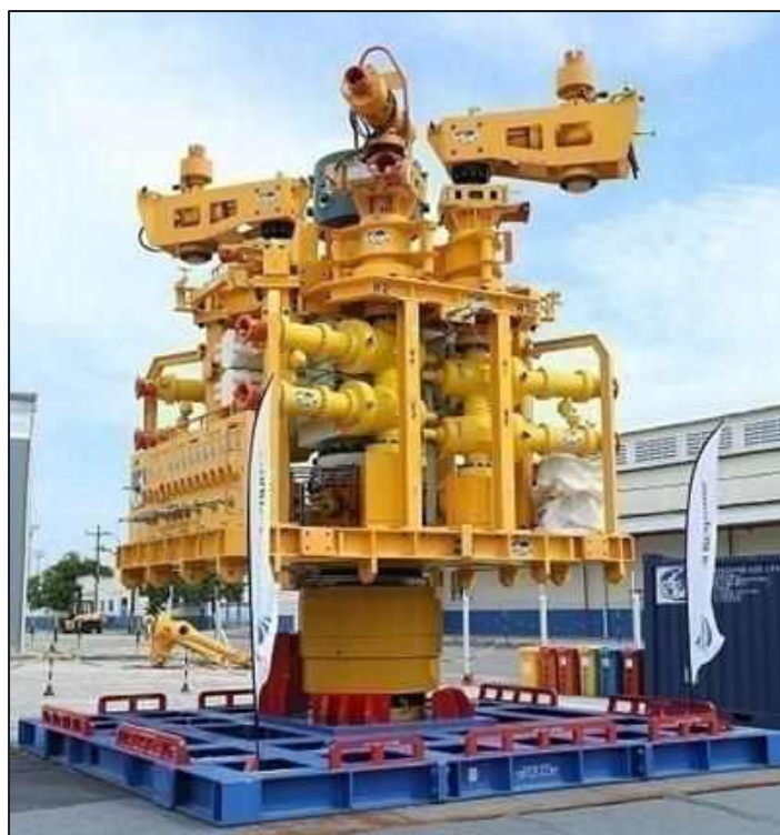
Figure 5-18: Example of an Oil Spill Response Limited Capping Stack.
