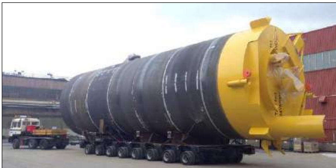
Figure 5-25: Example of a suction pile
