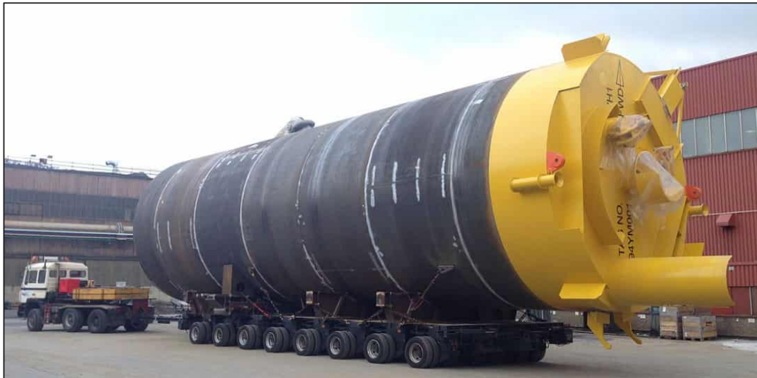
Figure 4-26: Example of a suction pile.
