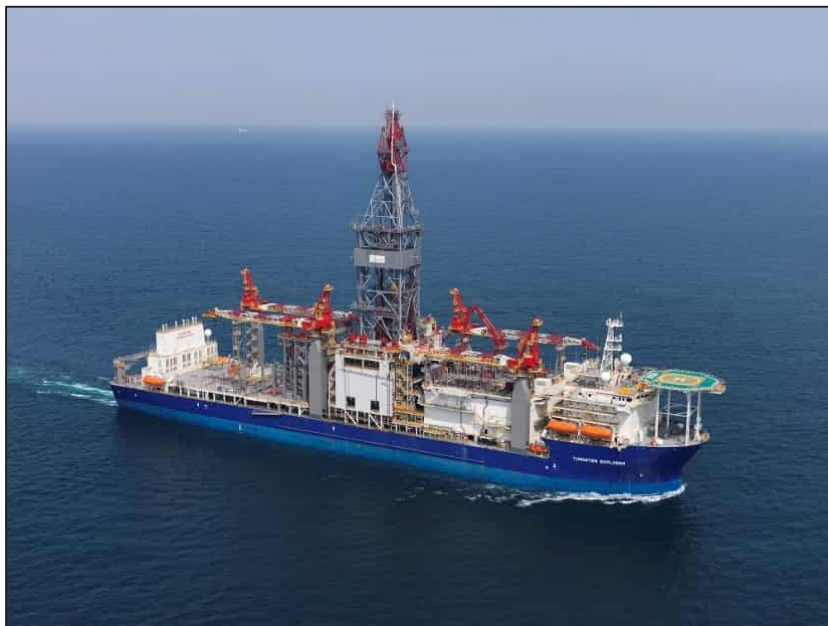
Figure 4-12: Example of a drilling unit (drill ship).
