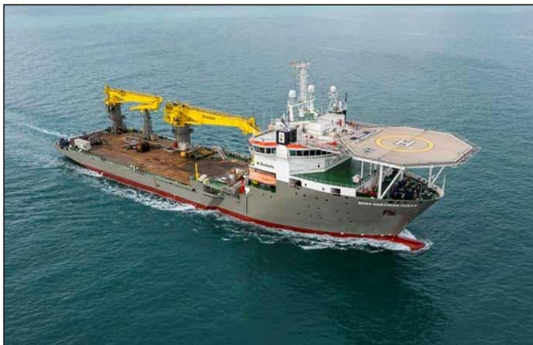
Figure 4-22: Example of a subsea construction vessel.
