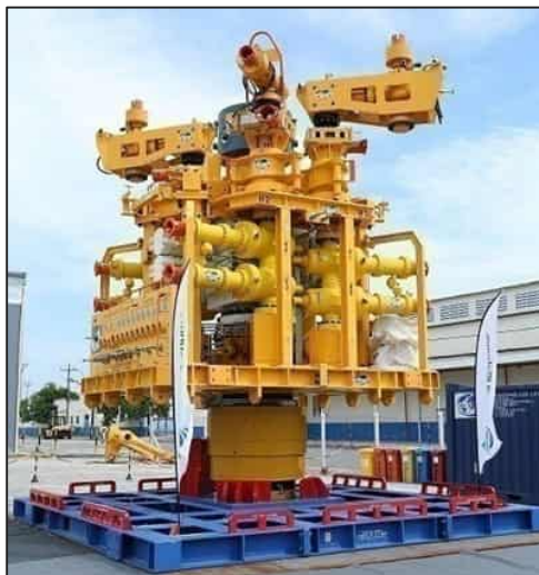
Figure 4-19: Example of an OSRL Capping Stack.
