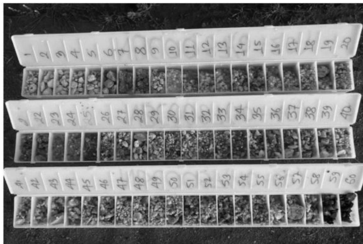
FIGURE 10 - ILLUSTRATIVE IMAGE OF RC DRILLING ROCK CHIPS (Photo taken from: https://www.marketindex.com.au/news/aldoros-pegmatite-intersections-at-murchison-look-encouraging )
