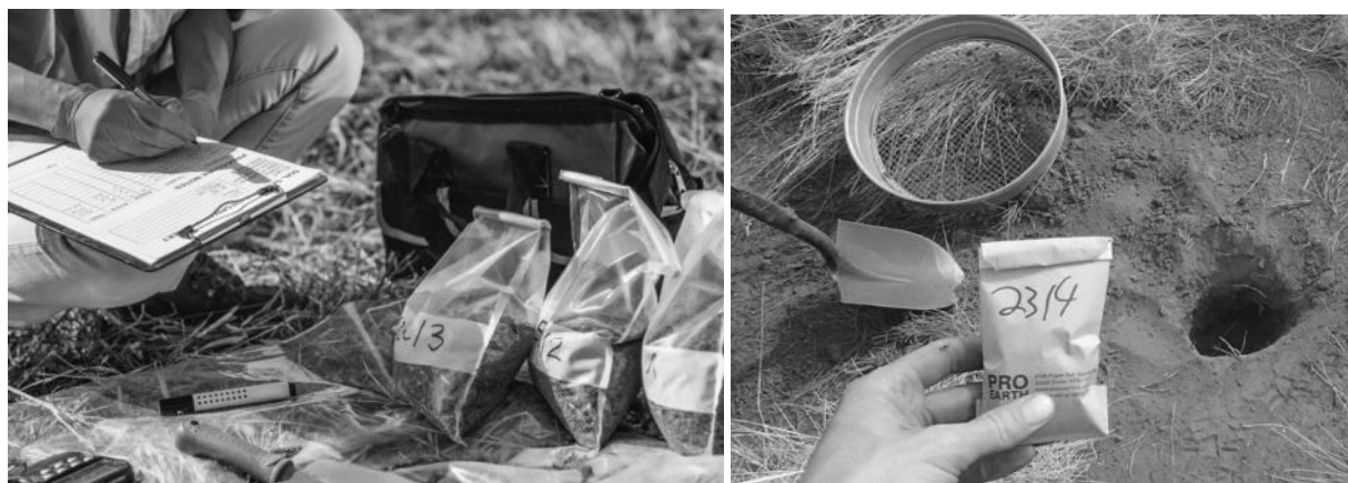
FIGURE 7 - EXAMPLES OF GEOCHEMICAL SAMPLING OF SOILS (Photo taken from: https://www.fishereng.com/post/b-understanding-geotechnical-investigations )
