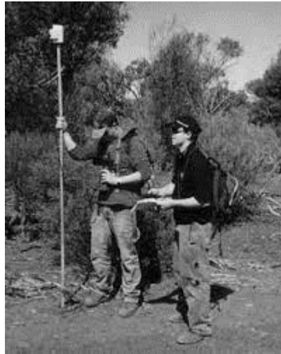
FIGURE 5 - ILLUSTRATIVE IMAGE OF A GROUND-BASED GEOPHYSICAL SURVEY WITH MAGNETOMETER (Photo taken from: https://irsl.ss.ncu.edu.tw/media/course/CI/SIO_9.pdf )
