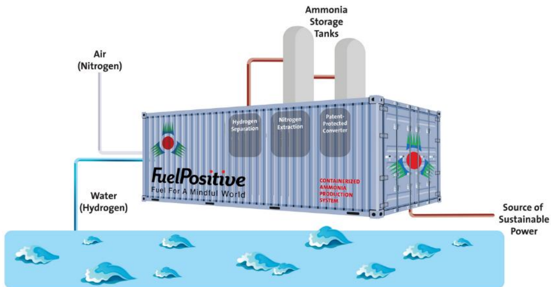
Figure 3: FuelPositive's containerized ammonia production system
