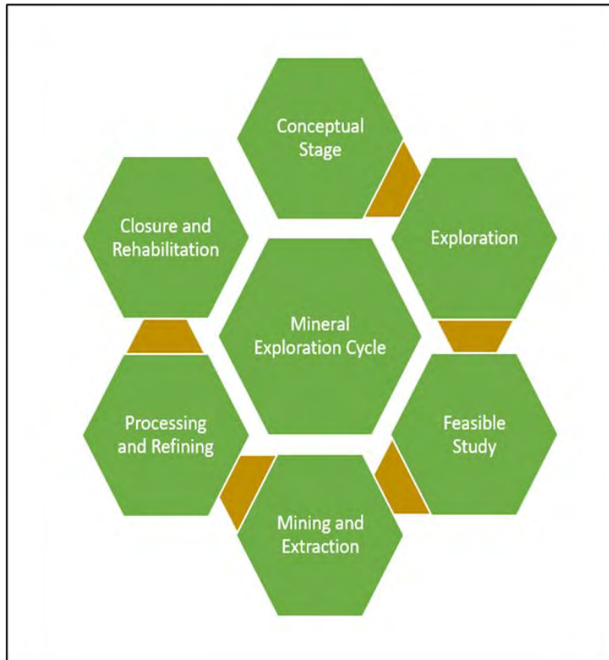
Figure 3-1: The Mineral Exploration Cycle, Adapted from the Association of Mineral Exploration, 2013
