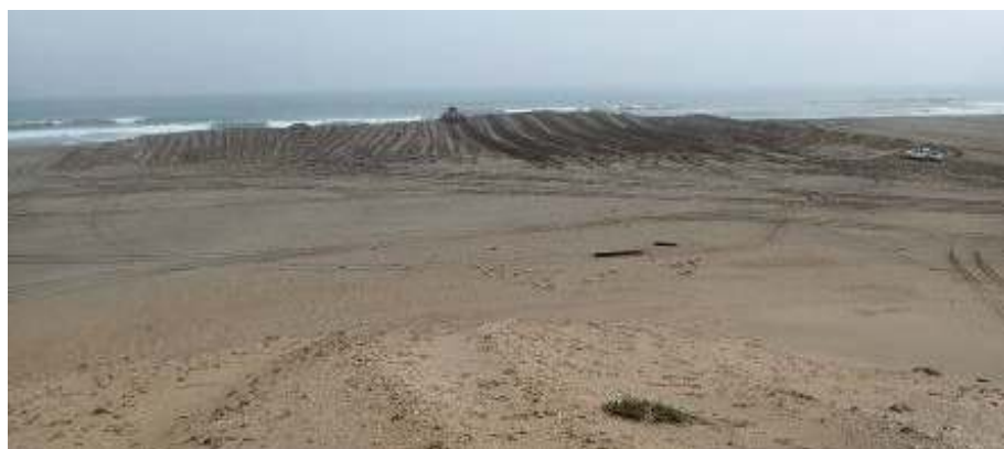
Figure 23. Northern block test mining: Stripping by dozer only (photo: Namdeb).
