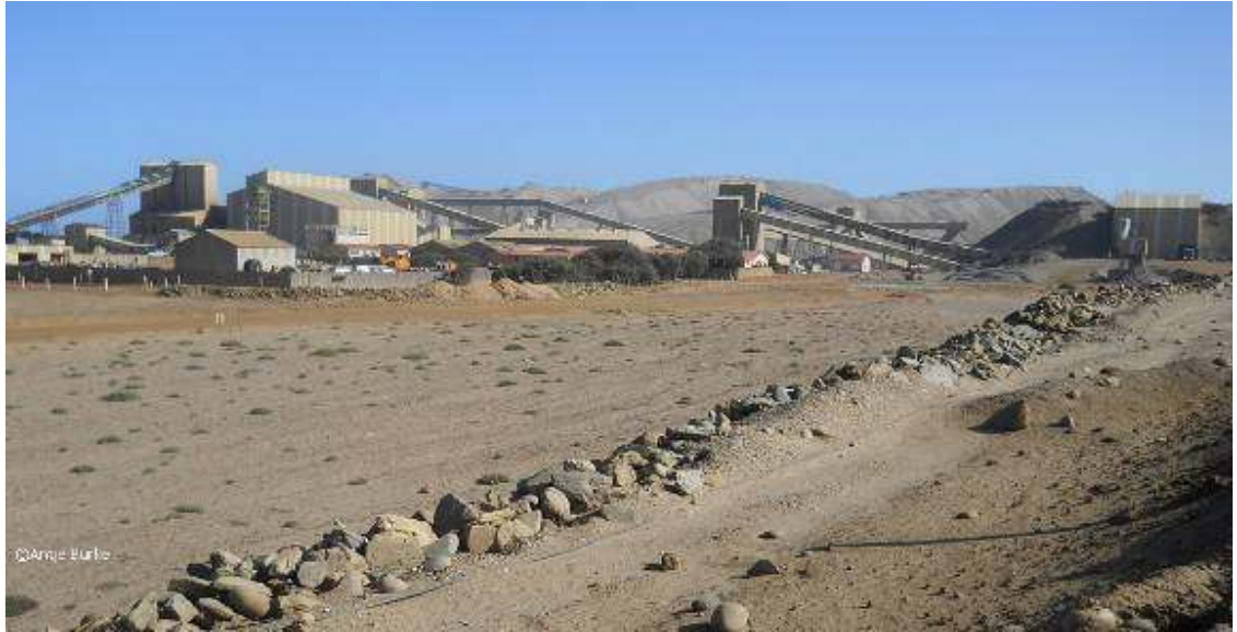
Figure 37. No.3 plant is a large processing complex with all typical components of a diamond processing plant such as crusher, scrubber, screens and Dense Medium Separation units.
