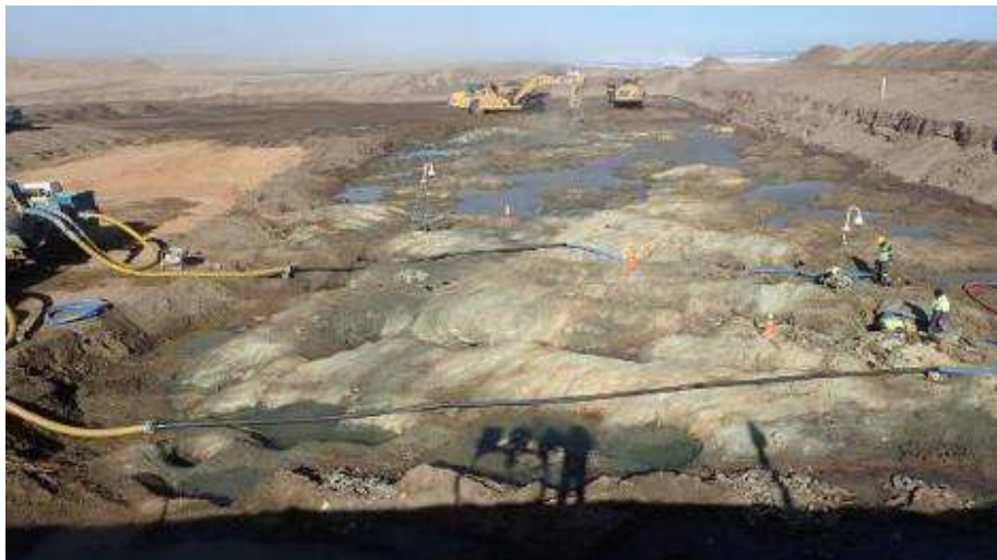
Figure 25. Northern block test mining: Fast, narrow strip mining (photo Namdeb).
