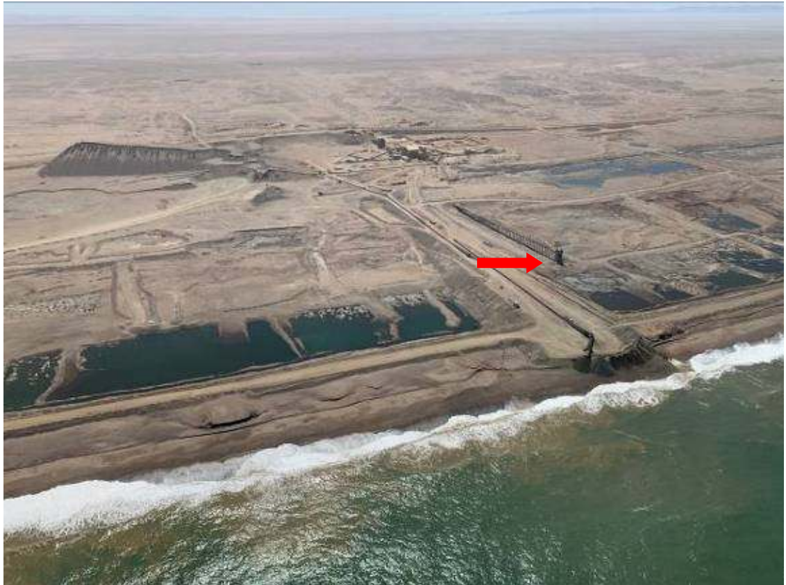
Figure 17. Conveyors transport material from overburden dumps as well as process plant tailings onto the beach to accrete the coastline, view from west to east at No.3 plant, in October 2020. The arrow indicates the former seawater intake tower which was the position of the former coastline some years back (Photo: Namdeb).
