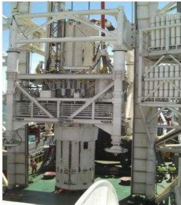
Figure 11. The 2.5 m diameter drill bit within the drill frame structure.
