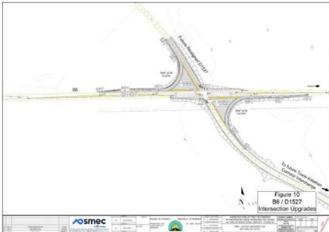
Figure 6 – Possible Slip Lane and D1527 stop sign intersection upgrade design plan (Source: (Innovative Transport Solutions (ITS), 2025)
