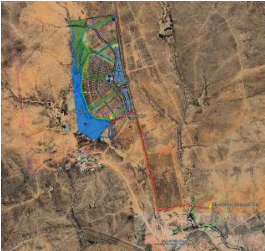
Figure 11 - Phase 1 Bulk Sewer Infrastructure (Source: WCE, 2026)
