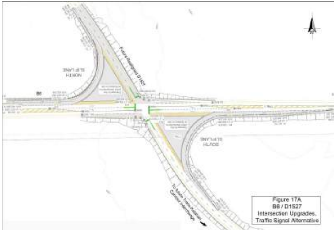
Figure 7 - Possible traffic signal alternative intersection upgrade design plan (Source: Innovative Transport Solutions (ITS), 2025)
