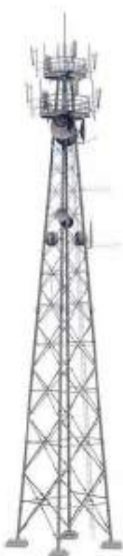
Figure 3 - A typical sketch of a lattice telecommunication tower
