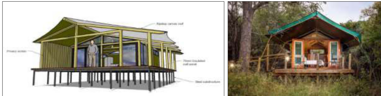
Figure 2-2: The specifications and illustrative photos of the external finishings of tented accommodation at the proposed Ekoto Tented Camp (source: Forgotten Valley Camps, 2024)
