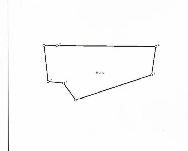
Corner points and map display: Projection: Geographic Datum: WGS84 The figure above represents parcel: 1 centimeter = 100 meters 200 UPI: EKOTO2100543 scale: 1:10 000 Size: 49.3 ha Decimal Degree Units: Corner points: Point Latitude Point Latitude Longitude Point Latitude Longitude Point Latitude Longitude Longitude 2 -18.82619 -18.82637 14.24172 -18.82801 14.24292 -18.82276 14.23983 14.24017 3 5 -18.82573 14.25059 -18.82302 14.25108 -18.82279 14.24114
