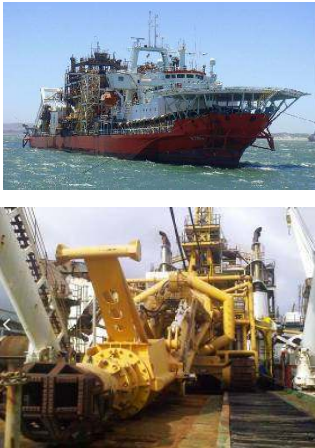
Figure 6: A typical mining vessel (above) and seabed crawler (below)
