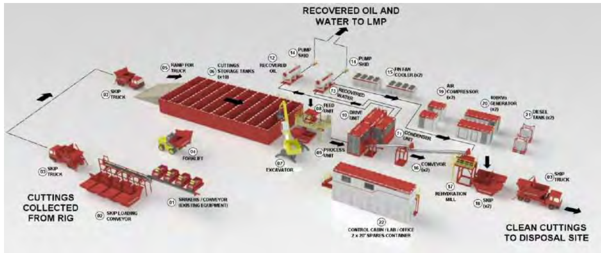
Figure 6: General layout of a Cuttings Treatment Facility
