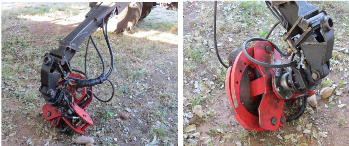
Figure 9: Small hydraulic buncher cutter used at the cheetah conservation fund, Otjiwarongo
