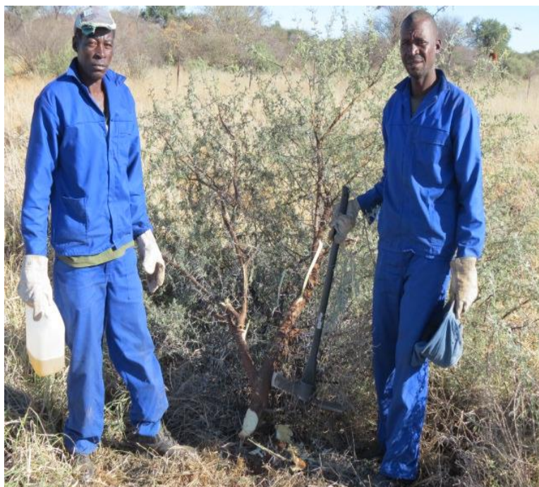
Figure 3: Manual bush pick used here for sickle bush clearing (courtesy Roads Authority of Namibia)
