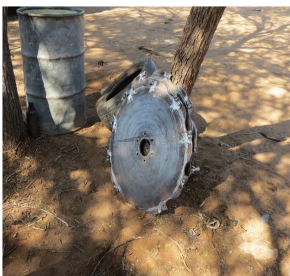
Figure 7: Repaired blades with new cutter for turbo saw (courtesy Forklift & Allied, Windhoek)
