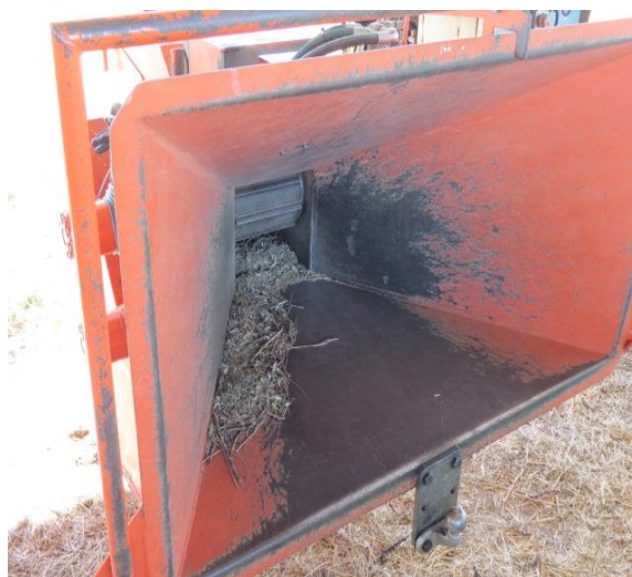
Figure 21: Small PTO driven chipper (left) Intake hopper and feeder rollers of chipper (right) (courtesy of Georg Fredrich, Witvlei)
