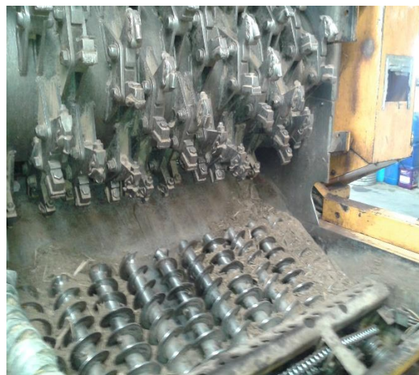
Figure 19: Grinder drum getting serviced
