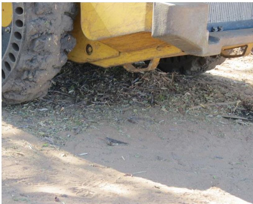
Figure 27: Note pieces of wood after machine compartment was cleaned out
