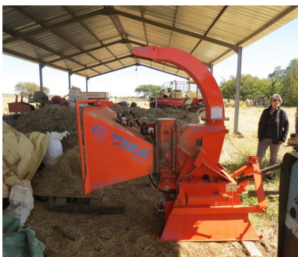
Figure 21: Small PTO driven chipper (left) Intake hopper and feeder rollers of chipper (right) (courtesy of Georg Fredrich, Witvlei)
