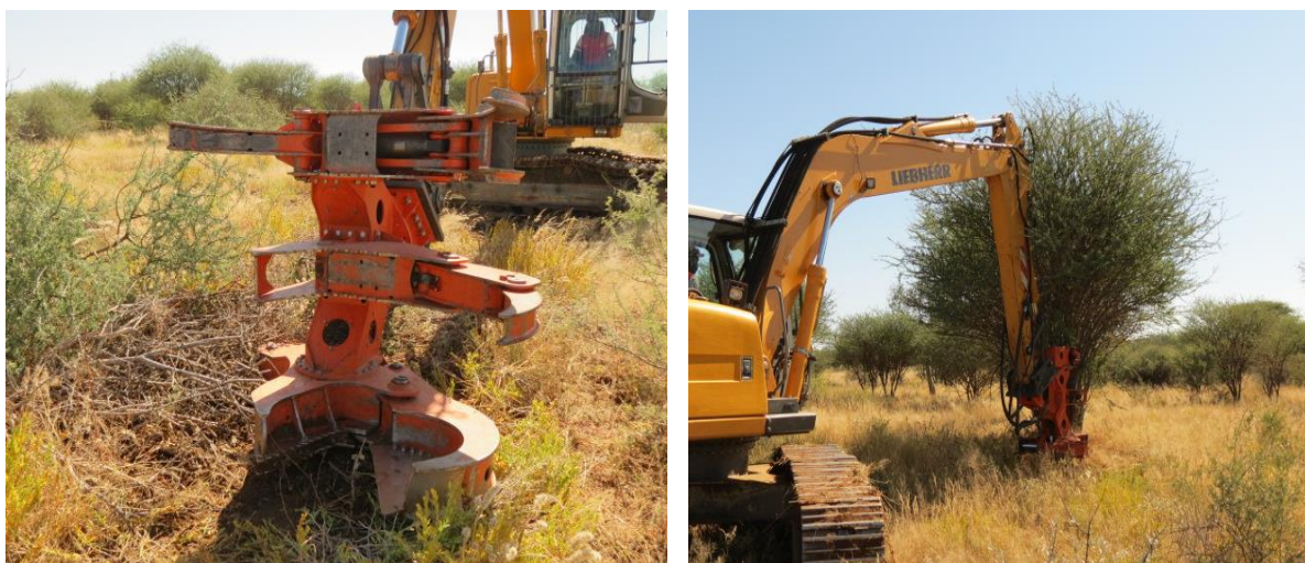
Figure 10: Hydraulic grab and cutter fitted to an excavator (left). Cutting a bunch of Acacia mellifera (courtesy Woodco, Okahandja)
