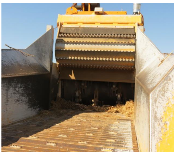
Figure 22: Large grinder infeed channel (courtesy TriCycle, Langebaan)
