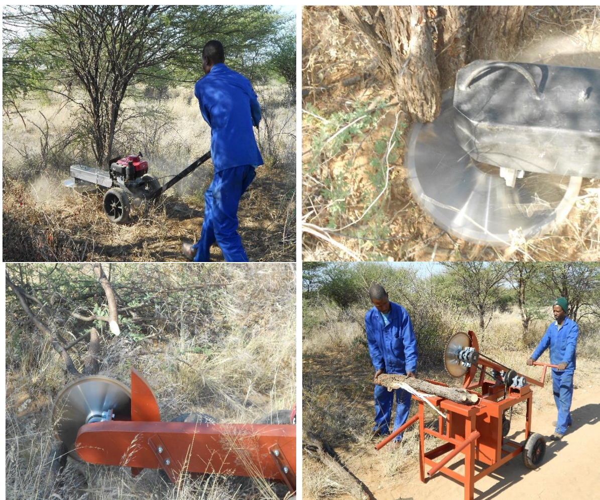
Figure 4: Trolley saws in action – horizontal saw tree feller (top) & Logger (bottom) (Courtesy Inventec, Otjiwarongo)
