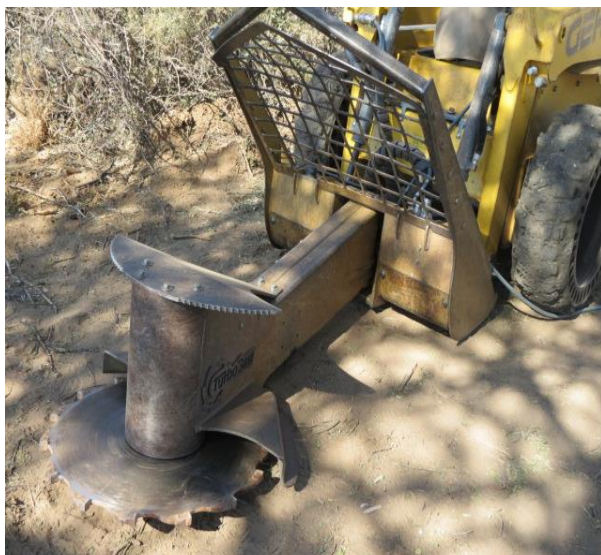
Figure 6: Gehl skidsteer with Turbo saw (Courtesy Callie Steenkamp, Kalkfeld)
