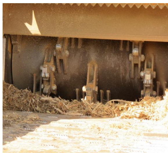
Figure 21: Small PTO driven chipper (left) Intake hopper and feeder rollers of chipper (right) (courtesy of Georg Fredrich, Witvlei)
