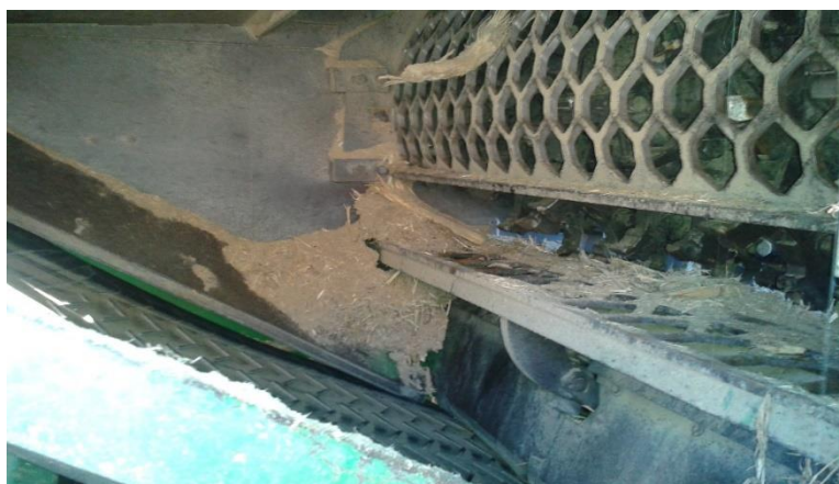
Figure 23: Drum screen with open gate and discharge conveyor (left) (courtesy TryCycle, Langebaan)
