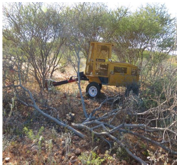
Figure 5: The “boscut” felling machine with hydraulic motor driven horizontal saw blade (Courtesy Peter Weder, Groot Aub)
