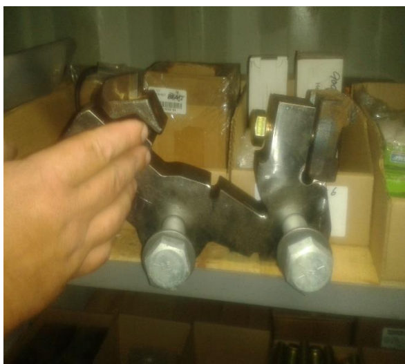
Figure 18: Grinder cutters assembled (courtesy WP Chippers, Worcester)
