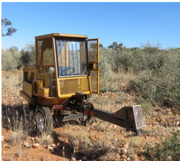
Figure 5: The “boscut” felling machine with hydraulic motor driven horizontal saw blade (Courtesy Peter Weder, Groot Aub)
