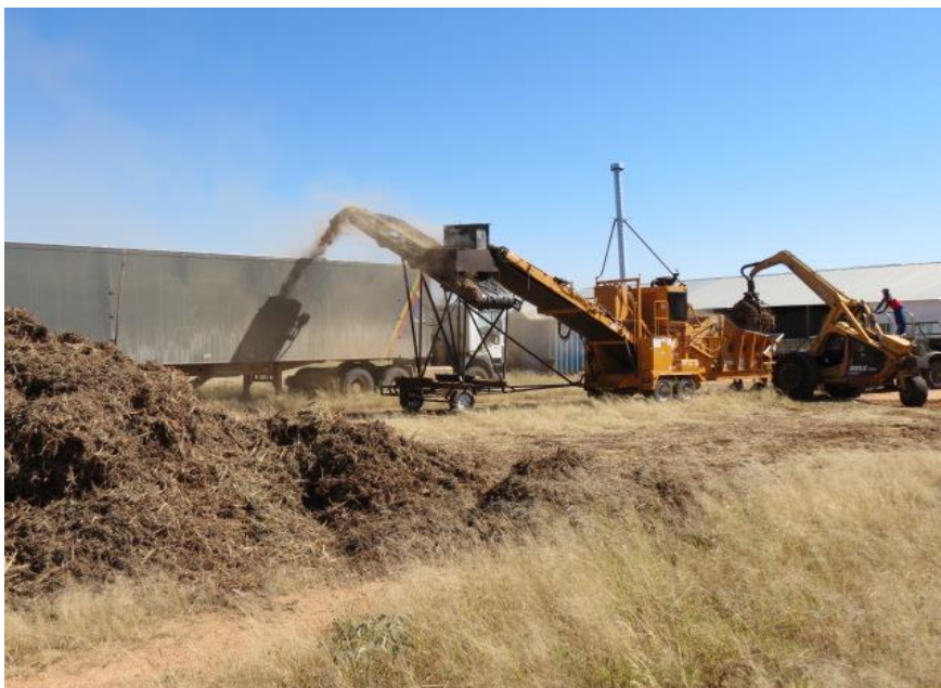
Figure 25: A commercial rechipping and transferring operation in action [Note large 110 m 3 road trailer in the background to the left] (courtesy WoodCo)
