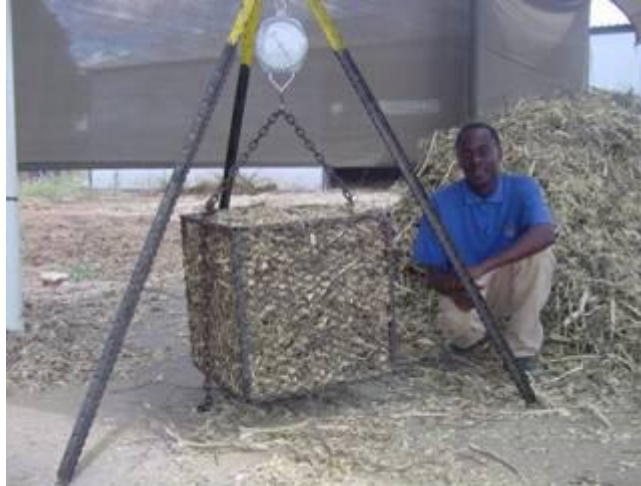
Figure 32. Measuring the wood chip density at CCF briquette factory in Otjiwarongo.
