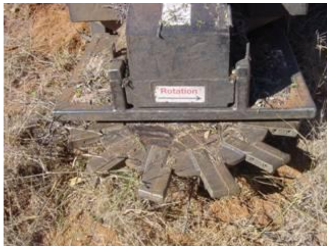
Figure 26. Rotary saw in the skid steer (photo by Arvo Leinonen).
