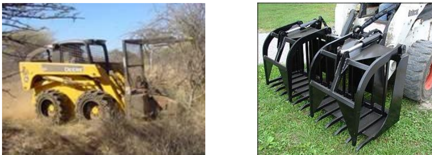
Figure 34. A skid steer (left) equipped with grapple for compiling the bushes (right).
