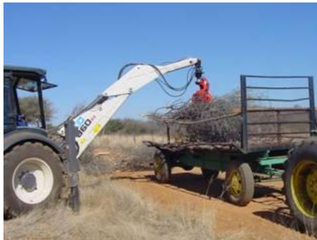
Figure 27. The bushes are loaded to the trailer by Nisula harvester head (photo by Arvo Leinonen).
