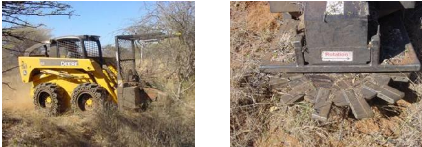
Figure 33. A skid steer (left) equipped with a rotary saw for felling (right).
