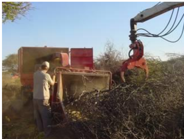
Figure 31. Feeding of the bushes to the chipper by Nisula harvester head (photo by Arvo Leinonen).
