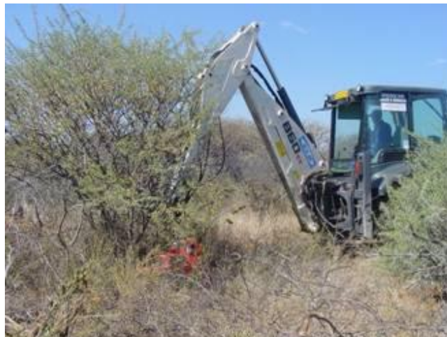
Figure 24. Nisula harvester head at work (photo by Arvo Leinonen).
