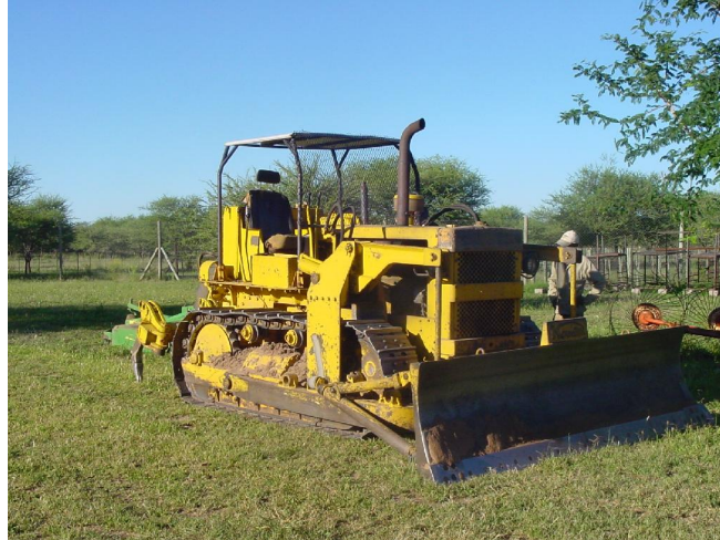
Figure 5. The bulldozer by which the strip roads are made (photo by Arvo Leinonen).
