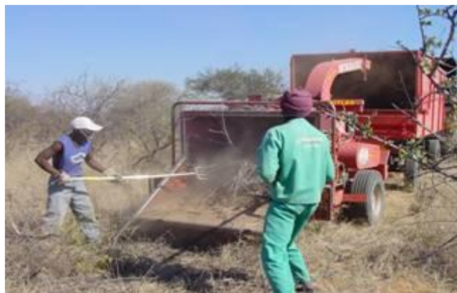
Figure 12. The bush chipping with Morbark Tornado Model 13 drum chipper at CCF in June 2007 (photo by Arvo Leinonen).
