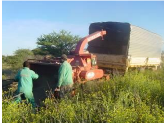
Figure 11. Bush chipping with Morbark Tornado Model 13 drum chipper at CCF in February 2007 (photo by Arvo Leinonen).
