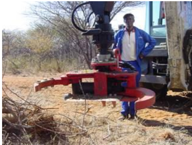
Figure 22. Nisula harvester head mounted on the boom in Terex backhoe loader. The pressing arms and cutting blade can be seen in the picture (photo by Arvo Leinonen).
