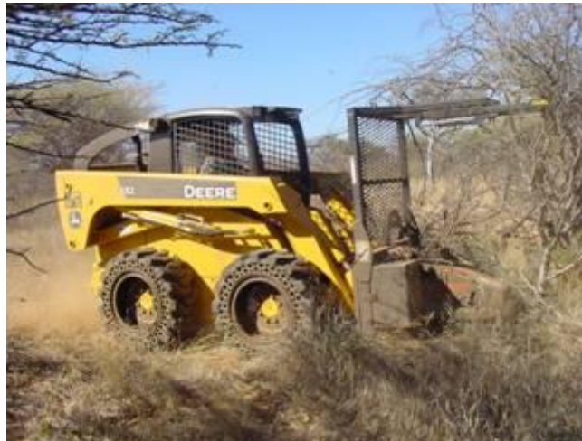
Figure 25. Skid steer with rotary saw at CCF in June 2007(photo by Arvo Leinonen).
