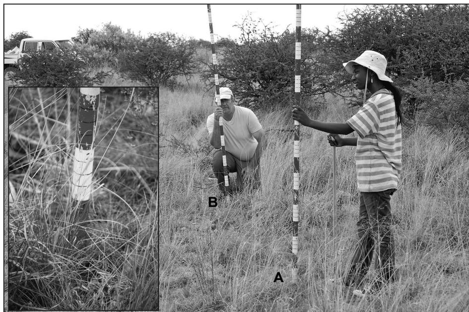
**Figure 1:** Method for taking a visual obstruction reading with a Robel pole (A) at a distance of 4 m, at a height of observation of 1 m (here, observation height is measured with a secondary Robel pole; B). Inset shows visual obstruction of vegetation against a Robel pole with 1 dm colour divisions with 0.25 dm markings
