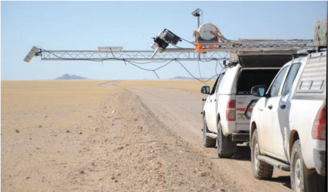
Figure 3: Characterizing LST homogeneity of the gravel plains between Gobabeb and Mirabib. The five TIR radiometers participating in the ESA FRM4STS field inter-comparison experiment (Göttsche et al. 2018) provided spatially resolved in situ LST along the driven track.
