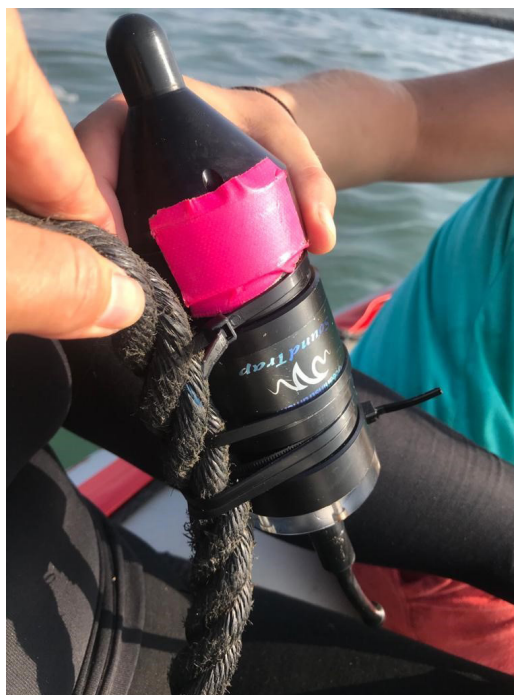
Figure 2: A SoundTrap 300HF (Ocean Instruments Inc., NZ) hydrophone used to make underwater recordings of the bottlenose dolphins ( T. truncatus ).
