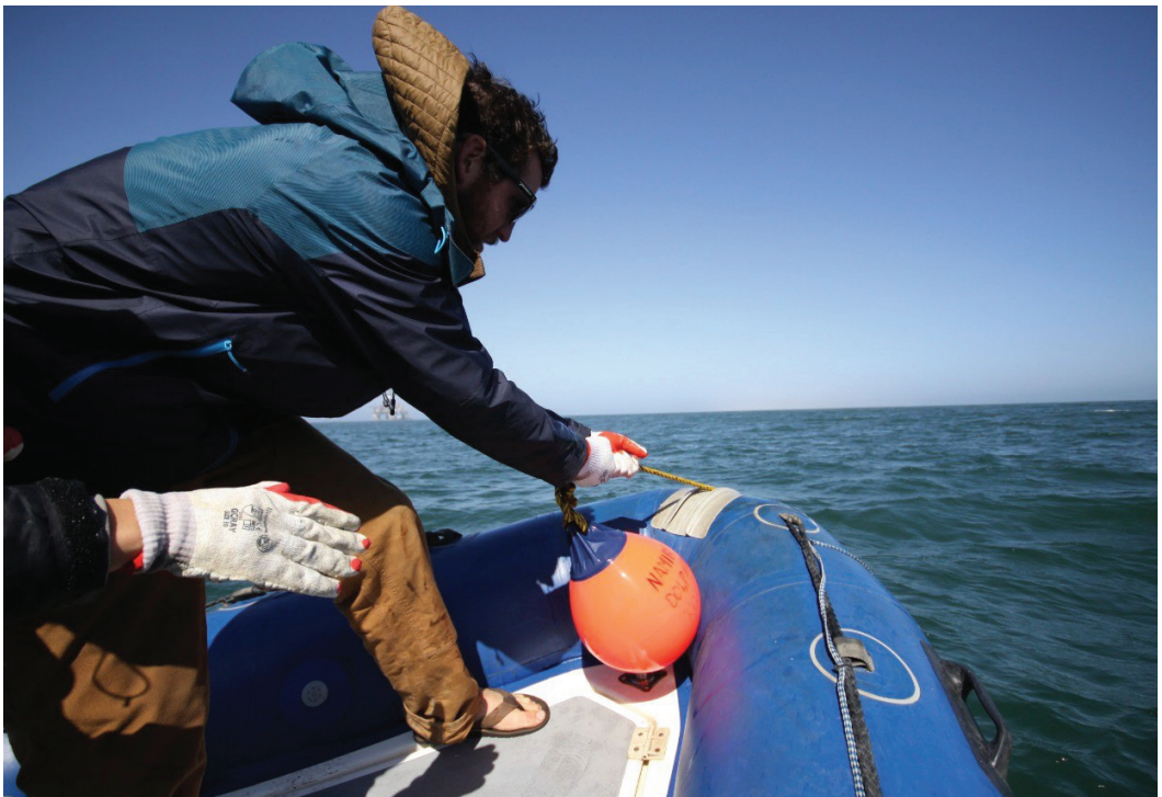
Figure 6: Jack Fearey is pictured here retrieving one of the SoundTrap recording devices in Namibia after a three-week deployment. The SoundTrap is attached to the rope/buoy system and weighted on the sea floor.
