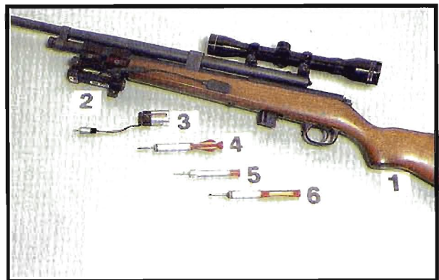
FIGURE 1: Immobilization equipment. 1. Model 171C Pneu-Dart rifle. 2. Laser Aim laser sight. 3. Charging cord for the laser sight. 4. 2 ml Palmer syringe. 5. 2 ml Pneu-Dart disposable syringe. 6. Syringe with reflective tape on the flight.
