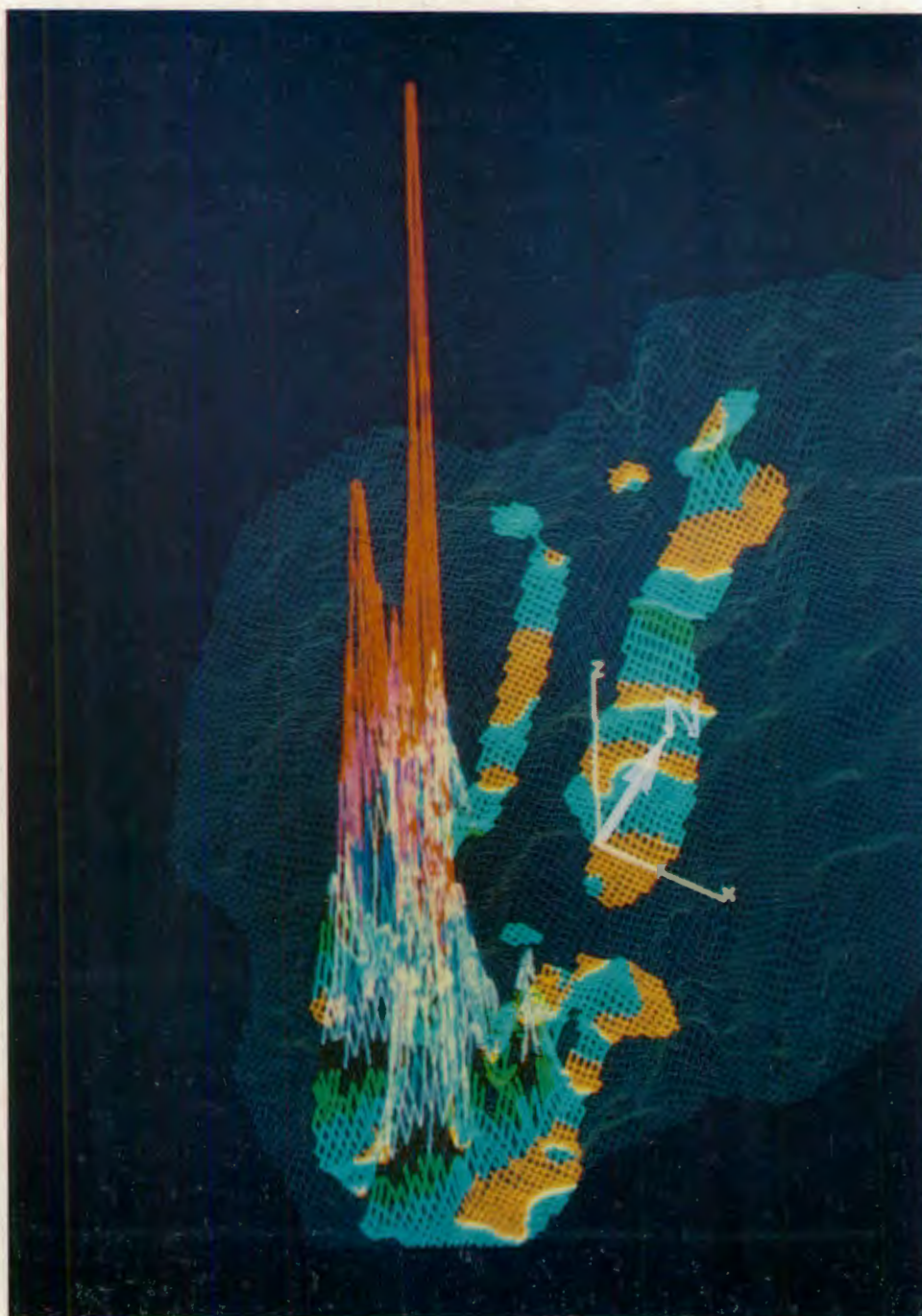
Figure 6.30. Diamond dispersal pattern shown by the variation of diamond concentration in the southern part of the Pomona claim. The variation of concentration is shown graphically, with peaks corresponding to high diamond concentrations. Colour coding of the diamond concentration contours are, shades of:
