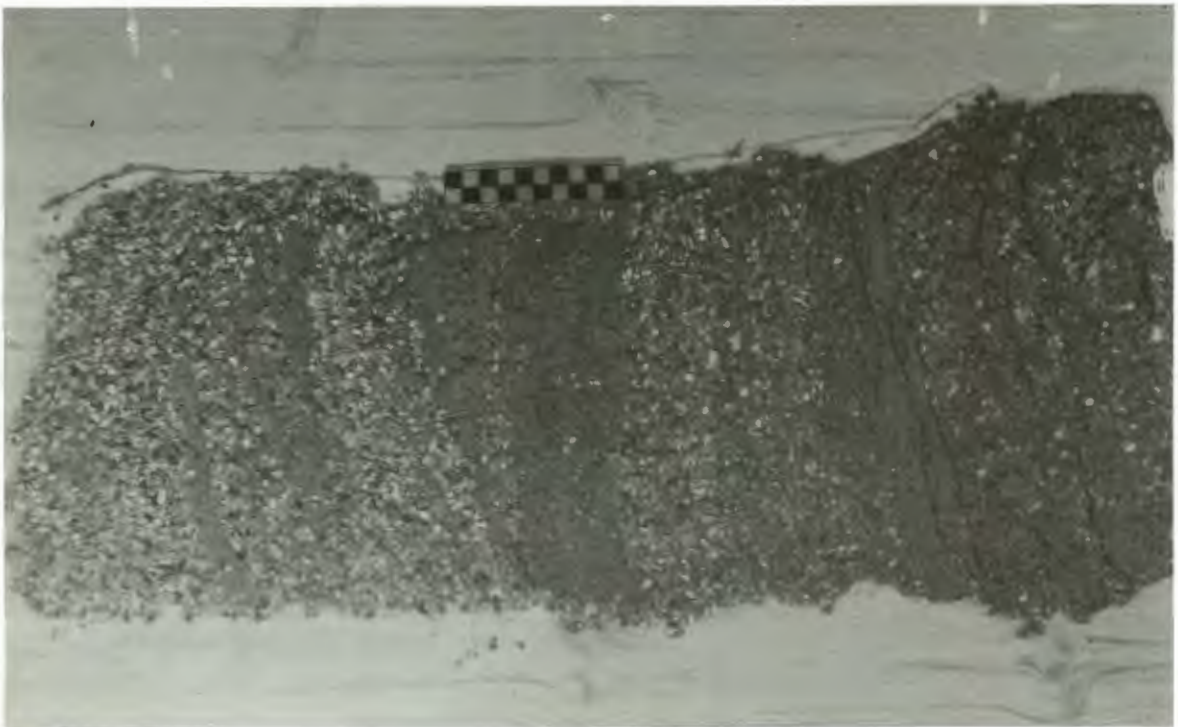
Figure 4.47. Cellulose acetate peel showing the stratification of the stoss slope deposits underlying the granules covering the surface. Crest of ripple is at the left end. Scale in cm.
