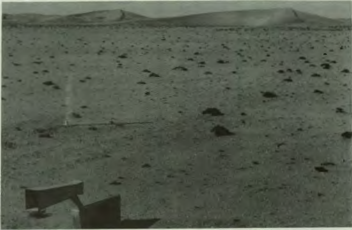
Figure 1.5. Sand trap site C. The venturi-compensated trap is seen in the foreground, and the compartmentalised, 1.83 m high perspex sand trap can be seen in the background. The barchan dunes on the horizon are about 28 m high, their crests have been slightly reversed by a northerly wind. Southerly wind flow is from top right to bottom left.
