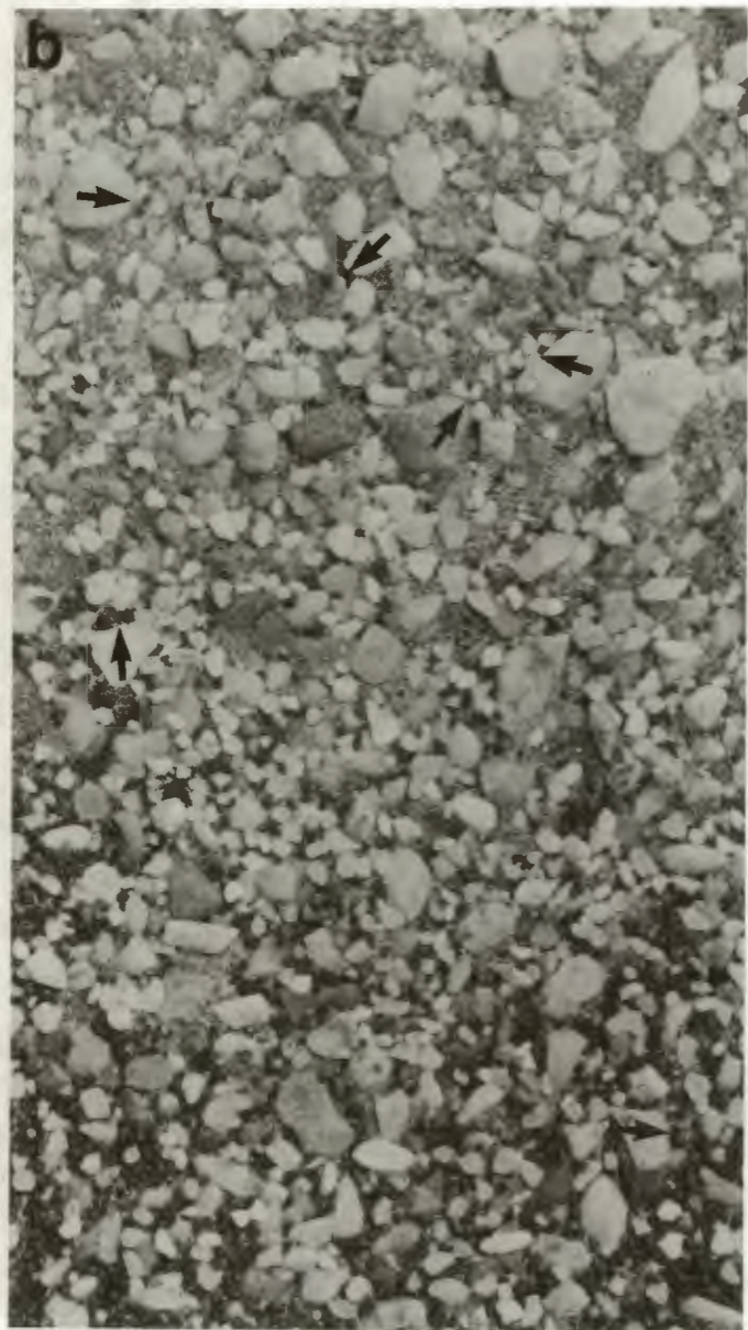
Figure 4.71. Stereo-pair of stone pavement taken during a northerly wind reversal on 22/09/87. (a) was taken about 5 minutes before (b). The arrows highlight the pervasive changes which effected the bed configuration as creep transport proceeded. The dark grains are the garnet bedload creep tracers used in the experiment on the stone pavement near sand trap site C. Note how some of the grains become lodged behind the immobile roughness elements.
