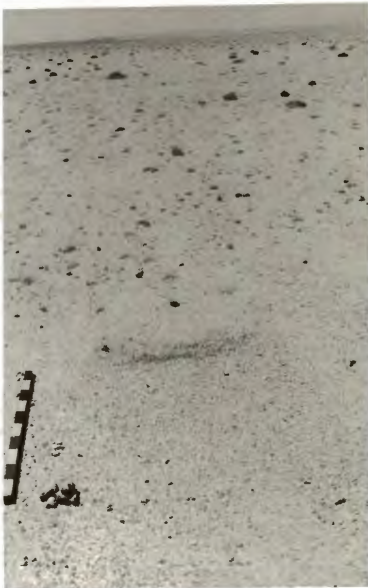
Figure 4.28. Dispersal of the garnet bedload creep tracers by aeolian processes. By 05/01/88 the initial line of garnet grains had been transported about 1 to 1.5 m to the north across the stone pavement. The original starting point is marked by a pile of stones near the scale. Southerly wind flow from bottom to top, scale 1 m.
