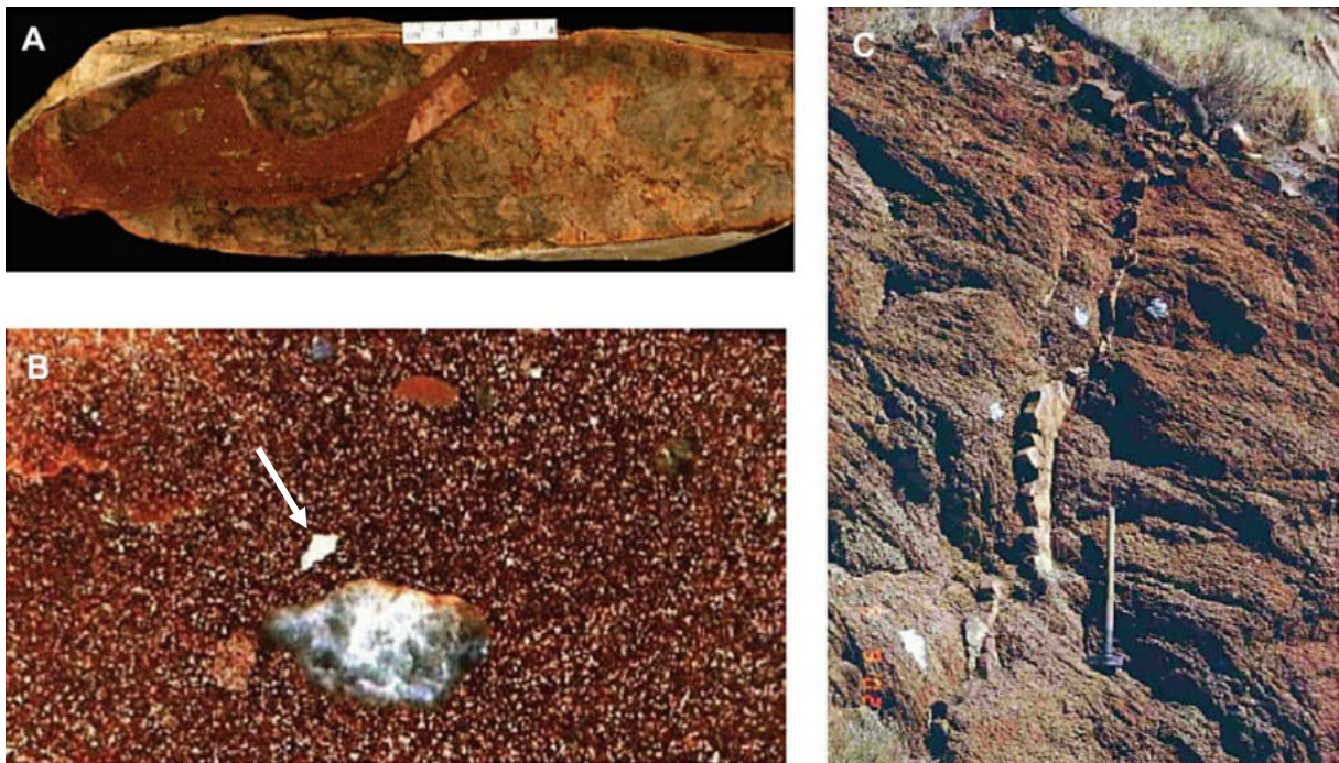
Figure 12. A) Clastic dyke of tuffitic sandstone with rhyolite clasts and numerous sericitised pumice fragments in brecciated Gamsberg rhyolite; B) Feldspar-rich clastic dyke (small light-coloured grains: feldspar and pumice fragments) in the Gamsberg quartzite with a large vein quartz clast, and smaller fragments of red rhyolite, devitrified volcanic glass (arrow) and silicified mudstone (image width: 6 cm); C) Clastic dyke cross-cutting Gamsberg granite
