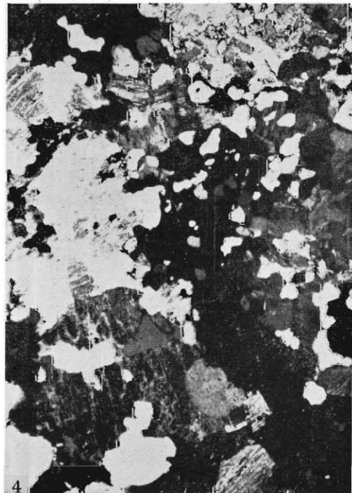
Figs. 1-4. Stages in the recrystallization of an acid tuff or lava characterized by the presence of aegirine-augite and by granophyric intergrowths of quartz and felspar. (T 67; T 12; T 13; T 8. Crossed nicols. Magnification \times 32 ).
