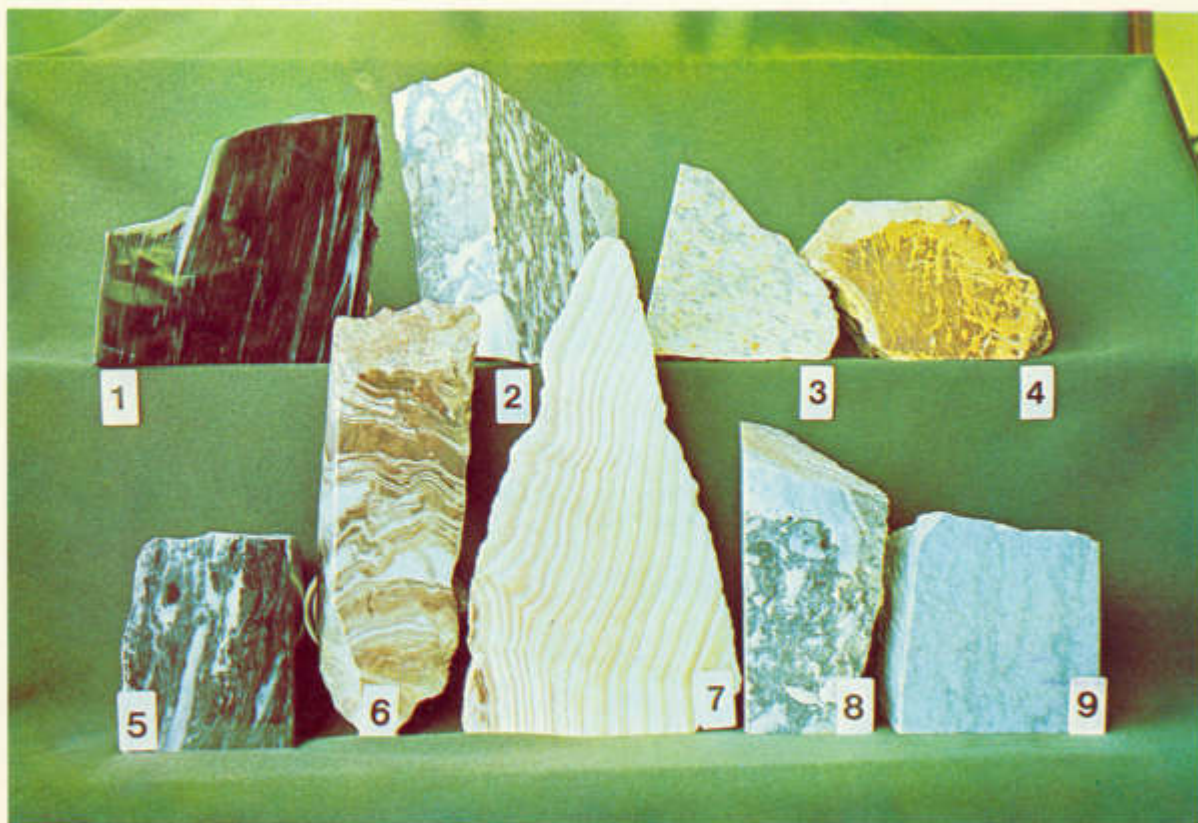
Plate X.—Various marbles from the Karibib-Swakopmund area (see text for details): (1) Black banded, (2) Grey flamed, (3) Nonidas green, (4) "Ewinde", (5) Black flamed, (6) "Antilope", (7) Aragonite, (8) "Leopard", (9) Dove-grey. The figures are 16 mm high (Photograph by the courtesy of the State Museum, Windhoek.)
