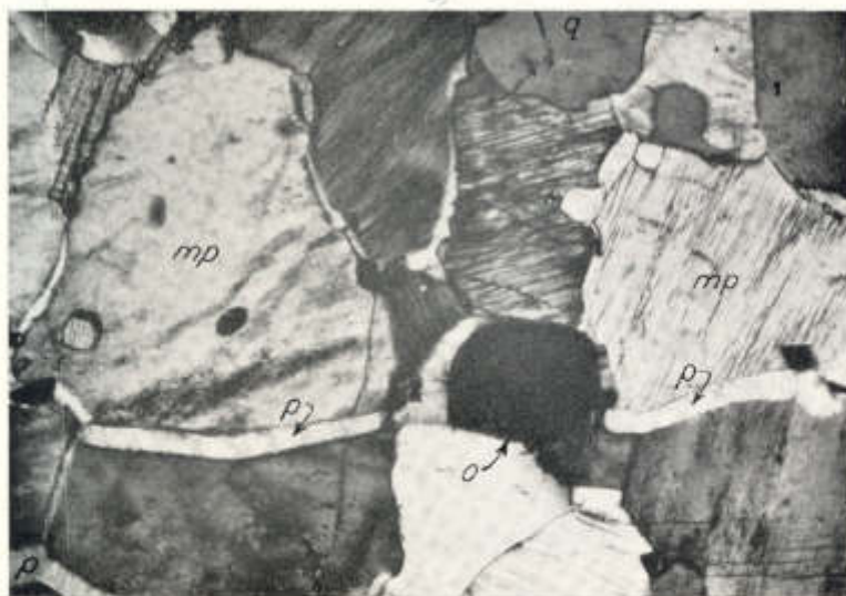
PLATE XVI.—Photomicrograph of rapakivi-type texture in red granite-gneiss at Louw's Claims (C. 1). (Sample SM 36.) q=quartz, p=plagioclase, mp=microcline-perthite, o=ore. Crossed nicols, \times 32 .
