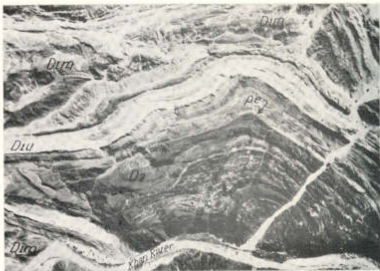
PLATE XIII.—Aerial photograph showing concordant pegmatites in Khomas Series. D 2 =Khomas schist, D 1m =tillite, D 1u =marble, pe =pegmatite.
