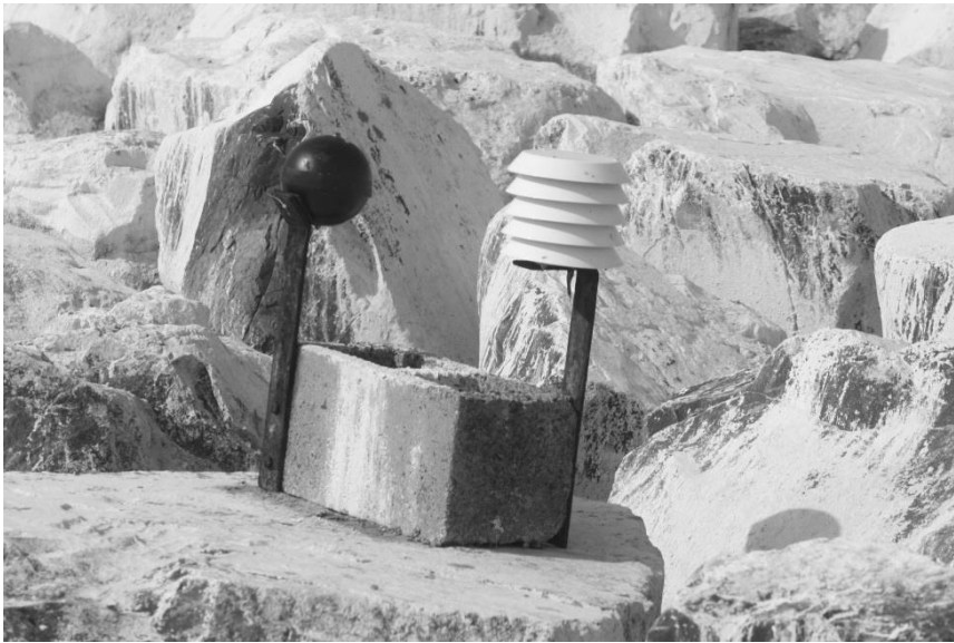
Figure 2.5. A black copper sphere and Stevenson's screen placed near the Robben Island colony
