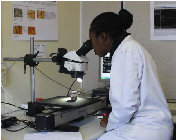
Figure 8: LinTab tree ring microscope for measuring age rings.
