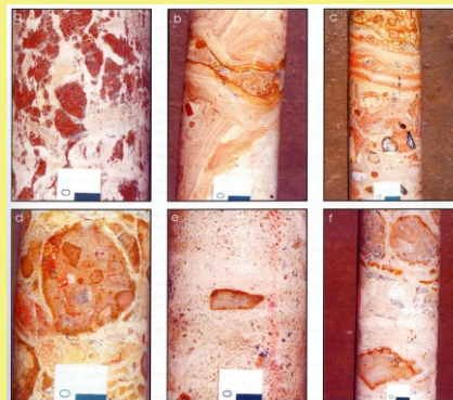
Diamond drill core of the Etosha Calcrete Formation
