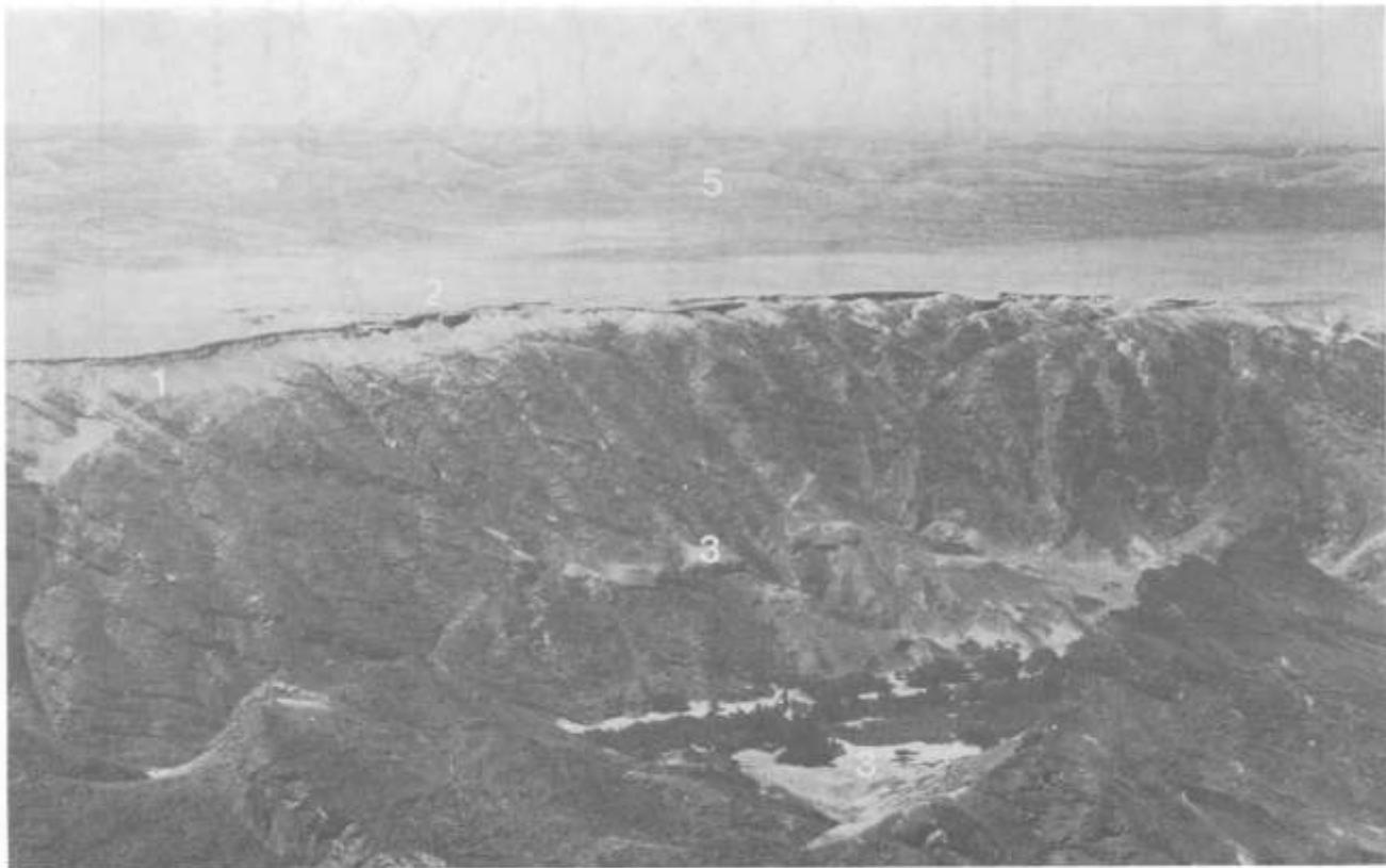
Figure 6: Oblique aerial view south-westwards over the Kuseb canyon at Gomkaeb, illustrating the salient features of the Cenozoic geology. 1: Erosion surface cut across Damaran schists 2: Tertiary deposits pre-dating canyon incision. 3: Quaternary terrace deposits post-dating canyon incision. 4: Modern Kuseb River. 5: Dunes of the main Namib Sand Sea. (after Ward, 1982).
