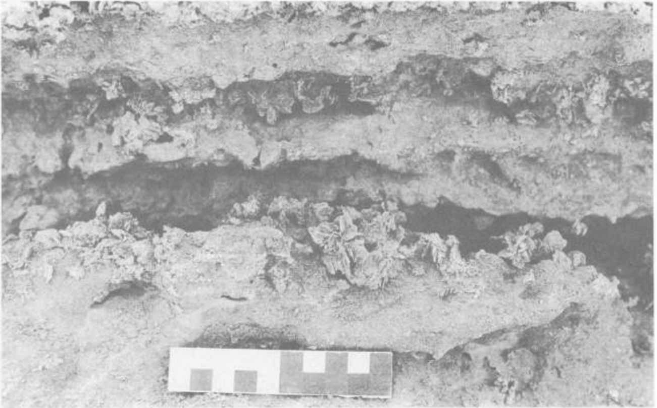
Figure 95: Gypsum crystal aggregates ("desert roses") forming a thin horizon in Awa-gamteb muds. Mile - 10 Reservoir area. Scale 10 cm long.
