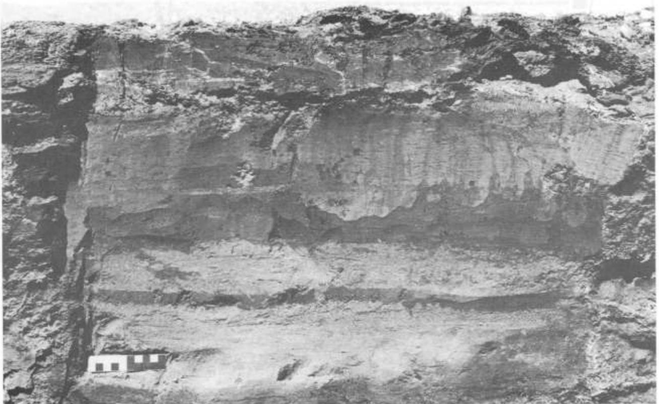
Figure 94: Dark clay layers intercalated with silts and micaceous sands in the upper part of the Awa-gamteb mud exposure near KP 110 beacon. Salt veinlets in uppermost clay bed. Scale 10 cm long. Section cleaned with a shovel gives appearance of soft-sediment deformation.
