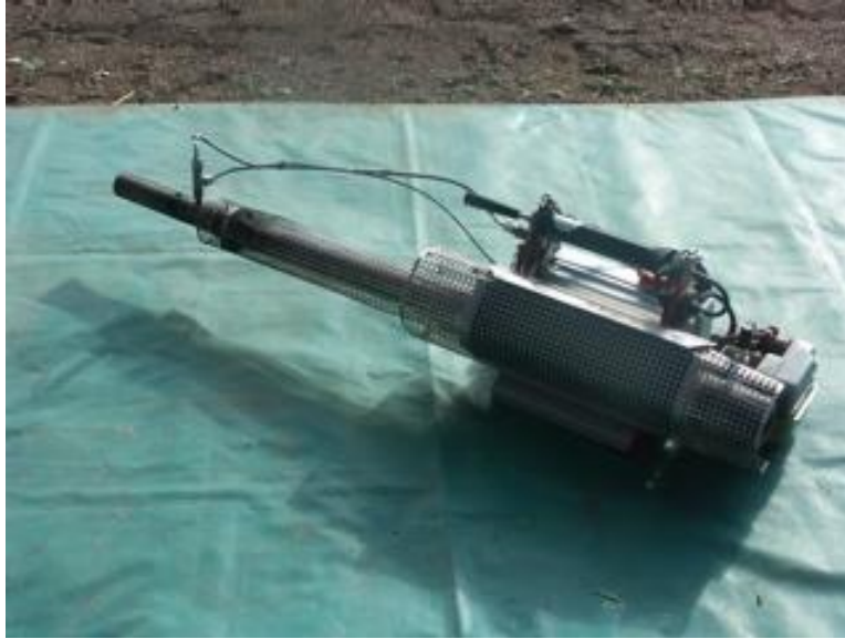
Figure 8. Motan Swingfog SN 50 disperser used to knock down insects from trees (Omaruru River, Namibia). (Photo: J. Theron, 2005)
