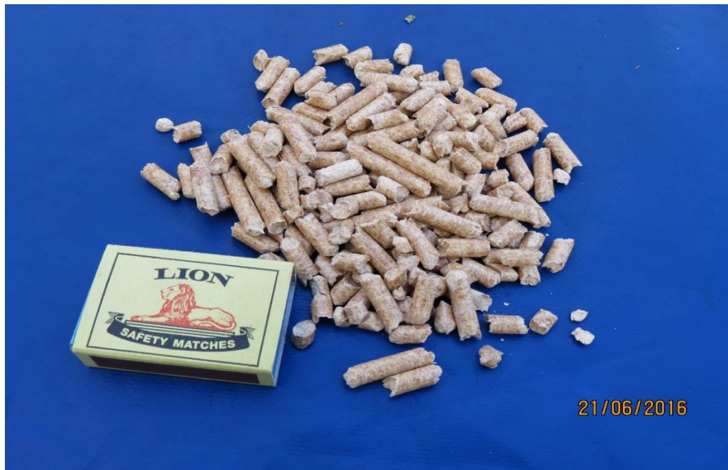
Photograph 32: White wood pellets ready to be used in a central heating system (Courtesy Italcotto)
