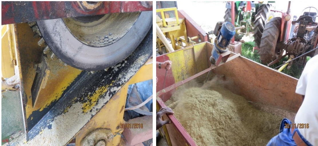
Photograph 9 & 10: Pelletising Operation (Larry Bussey)
