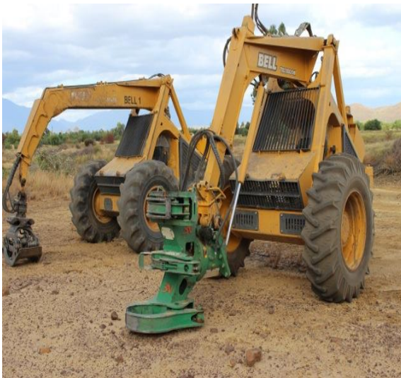
Photograph 6: Three-wheel logger (left) and logger fitted with a hydraulic cutter (right). Courtesy ABC Worcester
