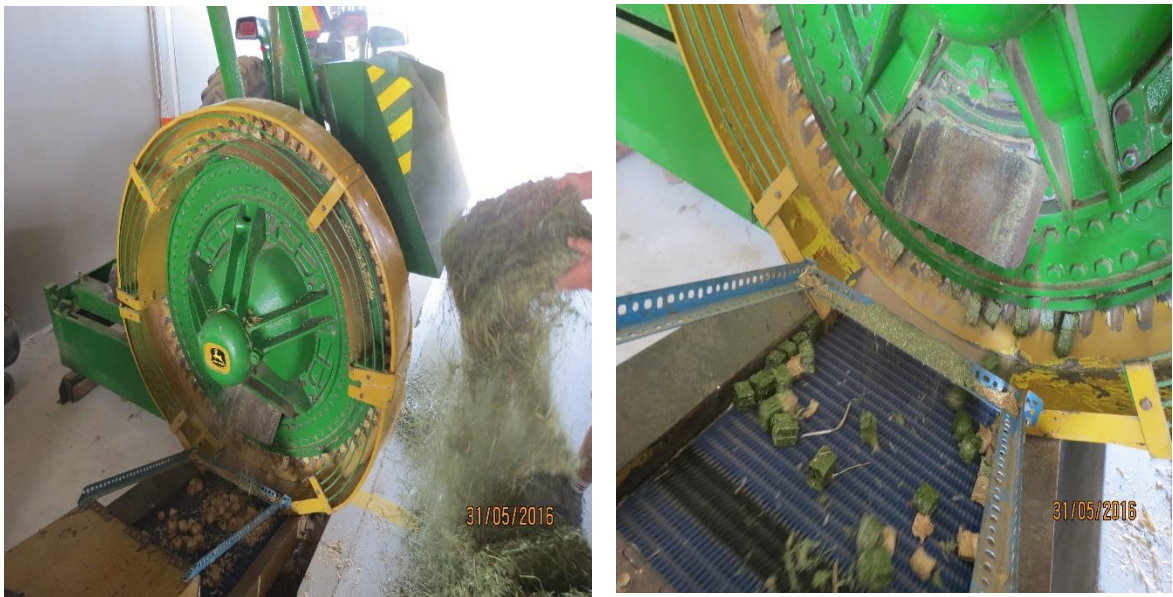
Photographs 11 & 12: Cuber machine in operation
