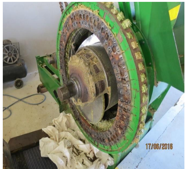
Photographs 13, 14, 15 & 16: A Cuber machine with its front wear plate removed to expose the 66 removable dies and eccentric press wheel
