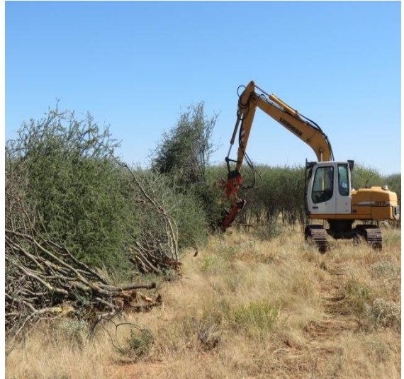
Photograph 7: Windrows being stacked with a hydraulic grab and cutter fitted to an excavator (WoodCo)
