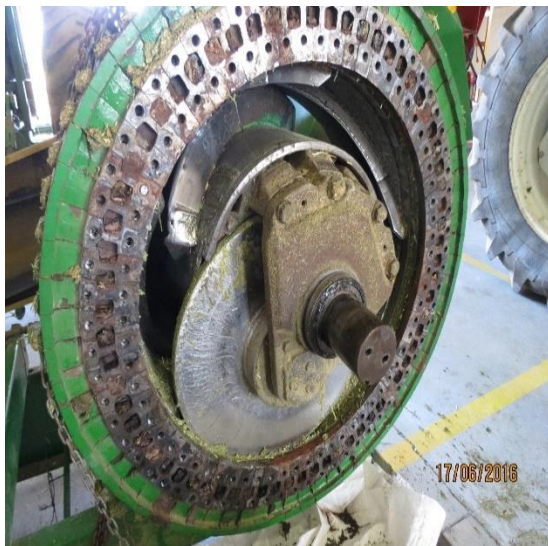
Photographs 13, 14, 15 & 16: A Cuber machine with its front wear plate removed to expose the 66 removable dies and eccentric press wheel
