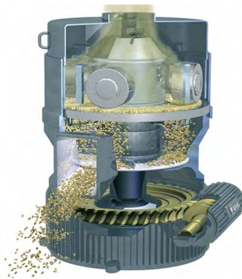
Fig. 5.19: Biomass pelletizing system [24]
