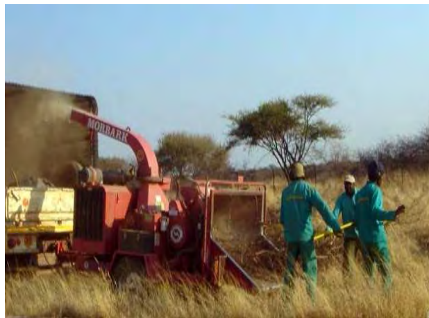
Fig. 5.12: Chipper for the production of biomass chips
