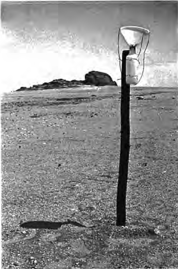
PLATE 1: Simple rain gauges were erected on the almost unvegetated plains to obtain the rainfall figures for this study.
