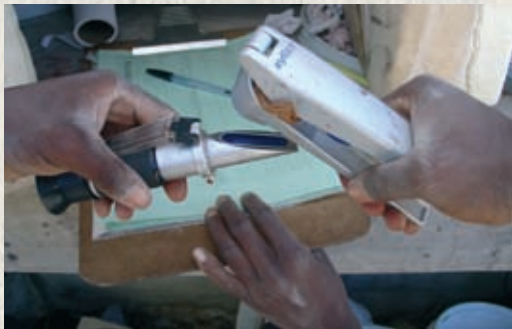
Figure 7. A drop of radish sap was squeezed onto a refractometer to measure the sugar and mineral concentration in brix.
